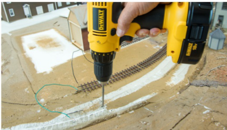
6 Power up. Lou used a long-shank bit to reach through the 4"-thick layout surface. He needed to drill new holes for the power feeders on the realigned track.
