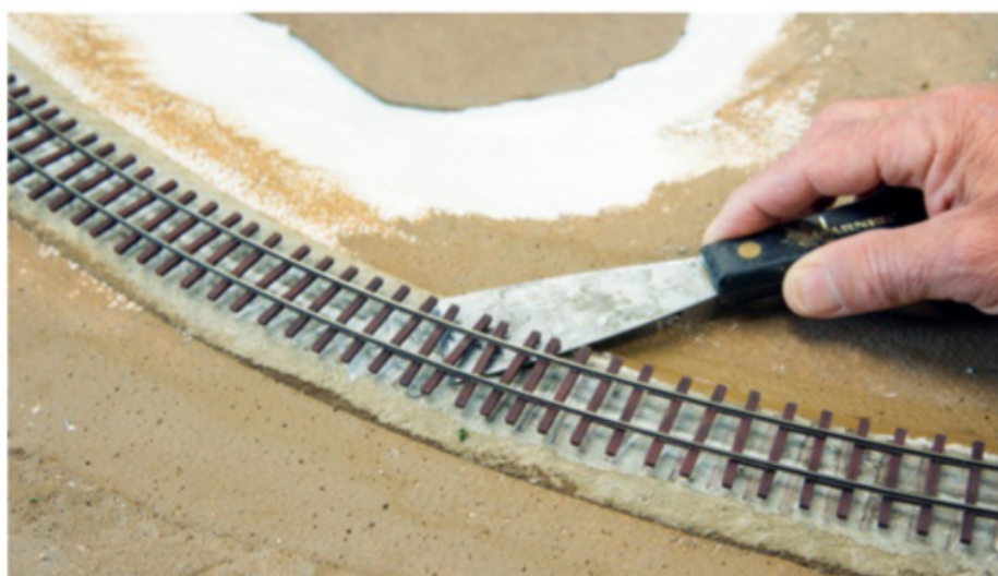
4 Away it goes. A putty knife finished the job and Lou was able to reuse the track. The Homasote roadbed, being a paper-based product, didn't fare as well.
