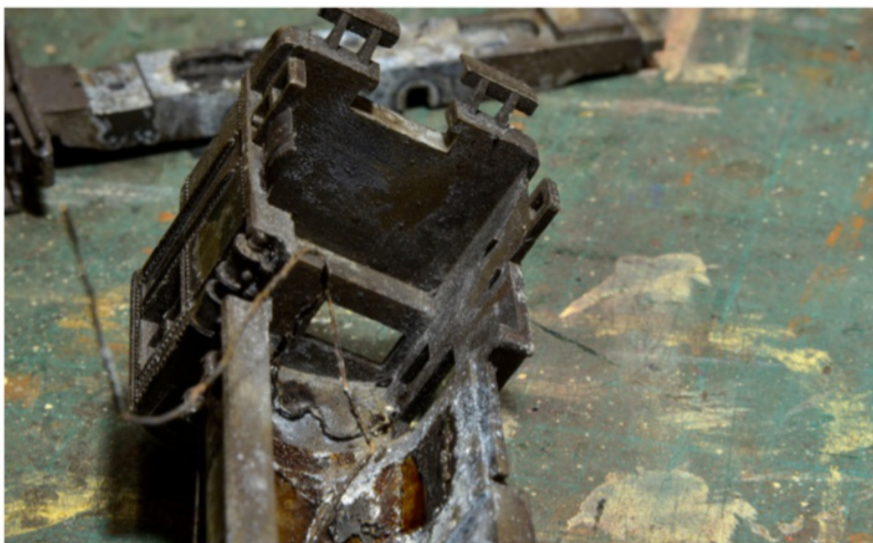
Even the wire to the headlight with its resistor survived the fire. The discoloration on the inside of the boiler hints at the extent of the damage.
