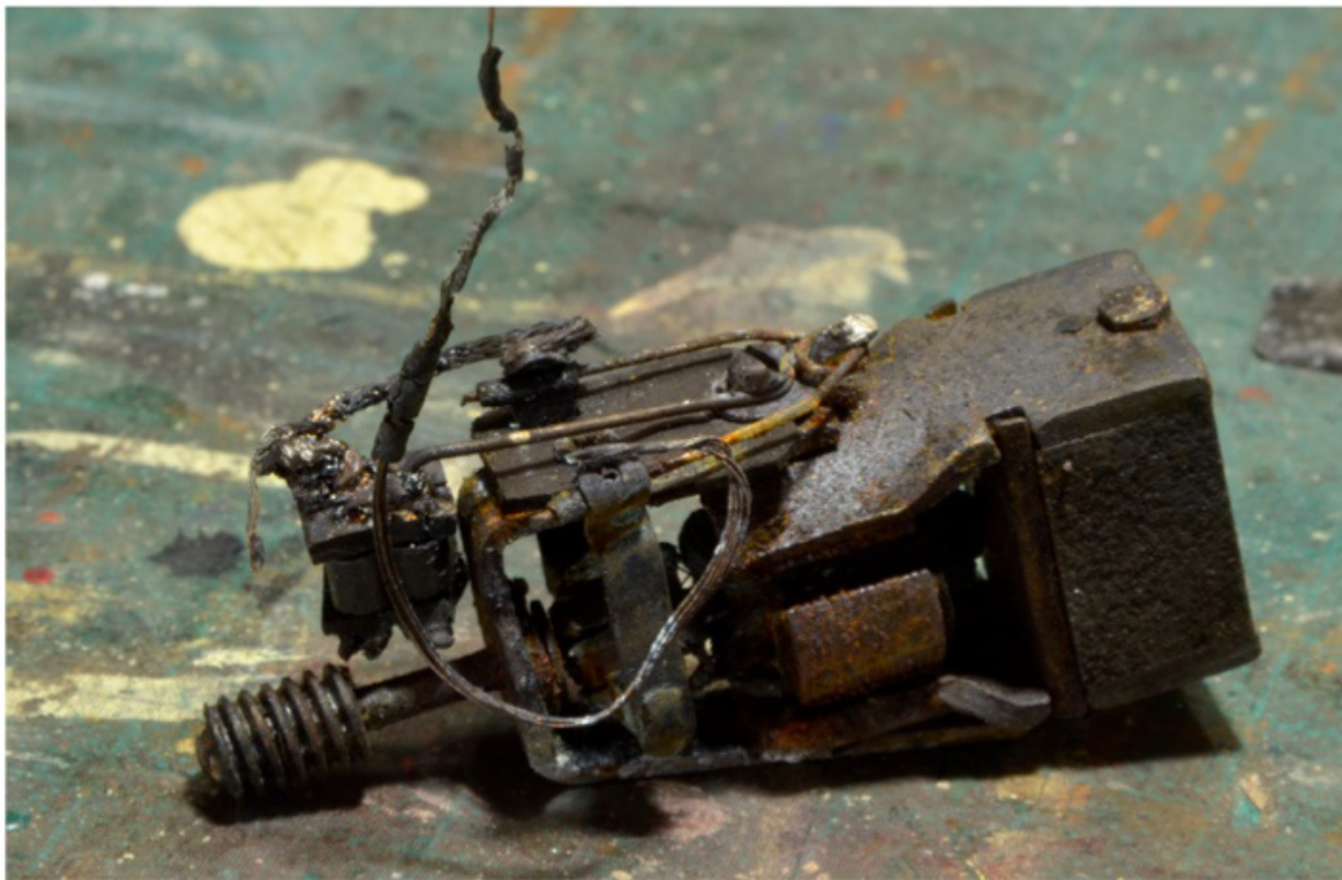
The vintage open-frame motor was beyond repair, but Kenichi was able to locate a duplicate of the original.
