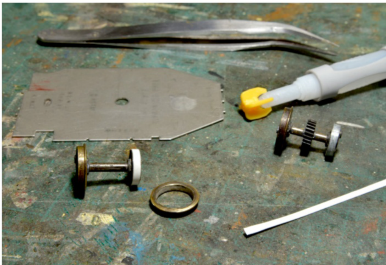
Kenichi created a new insulating driver rim from styrene. The original plastic had melted away.
