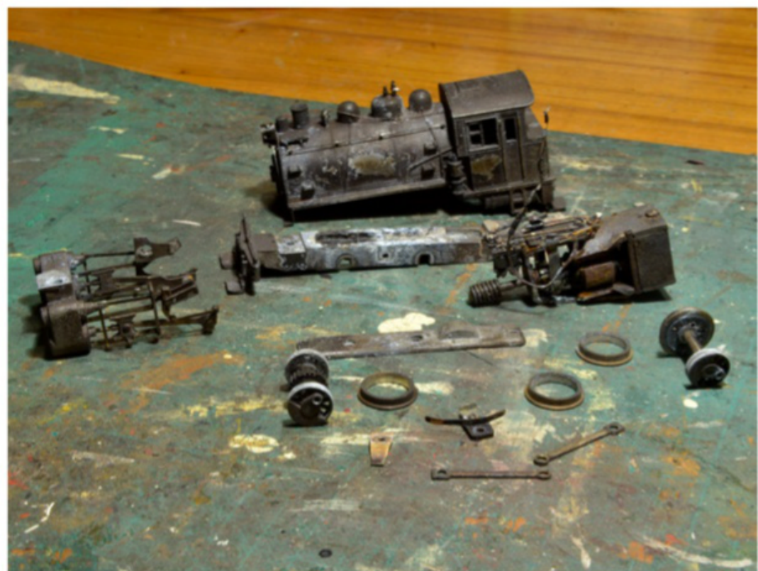
Kenichi started by disassembling the burned locomotive and assessing the damage.
