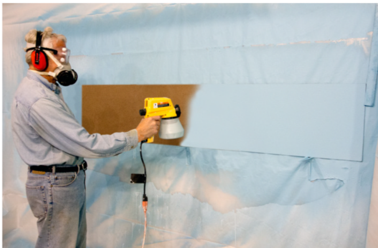
Fig. 1 Blue sky base. Gerry paints the base color. Hearing and respiratory protection are advised as the sprayer is noisy and produces airborne droplets.
