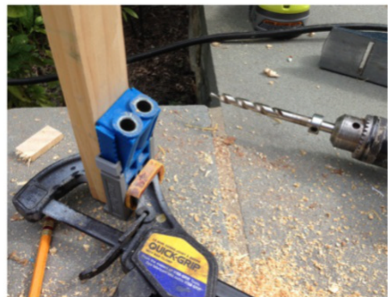
Bernie used a Kreg pocket screw jig to avoid inserting screws into end grain at butt joints. This tool isn't expensive and has many household applications.
