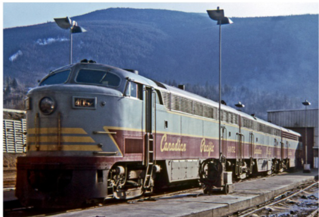
A Fairbanks-Morse A-B-A C-Liner set basks in the April 1967 sun between runs at the Nelson Diesel Shop. Their shared-cylinder, opposed-piston prime movers made a distinctive thrumming sound but created maintenance challenges for the lower bank of cylinders. Mike Barone photo
