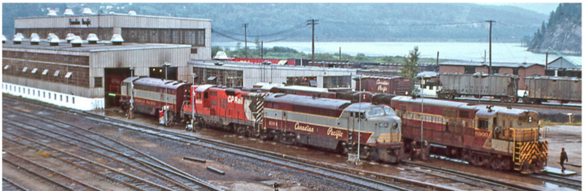
The Nelson, B.C., diesel shop in 1972 shows a preponderance of Fairbanks-Morse power plus a single Geep. Alco-designed power built by the Montreal Locomotive Works also frequented the area, making the location an interesting modeling era and site. Mike Barone photo
