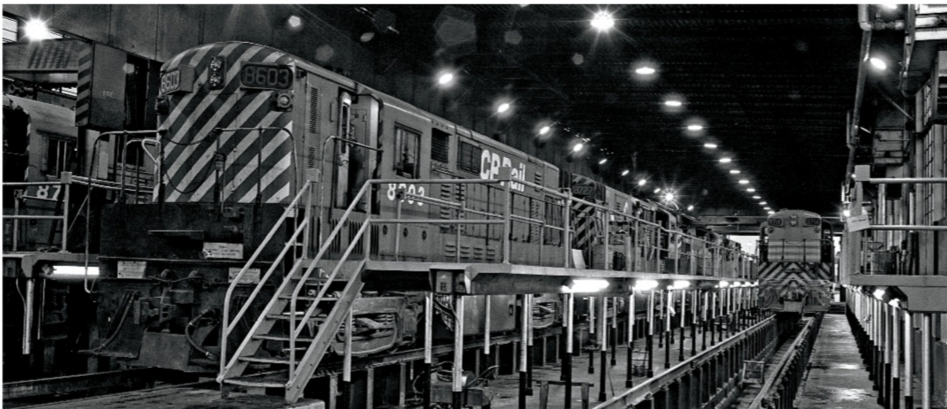
This black-and-white photo shows the inside of the Nelson Yard Diesel Shop. The platforms provide hood-unit walkway access, while the rails are supported on pedestals to allow easier inspection of the trucks. Mark Horne photo
