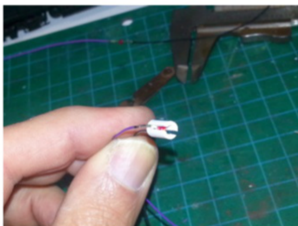
8 Marker lights. Louis mounted small, red light-emitting diodes (LEDs) into slots cut in styrene tubing for marker lights. The slots hold the LEDs' leads.
