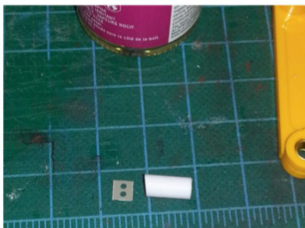
7 Headlight tricks. Louis drilled two no. 54 holes in a square piece of styrene to simulate the twin sealed-beam headlight mounted in the door.
