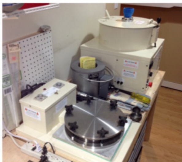
10 An entry-level spin-casting system. The steel circular disk in the foreground is the mold vulcanizer. The spin-casting machine is in the rear. In the middle is the small electric metal melting pot.
