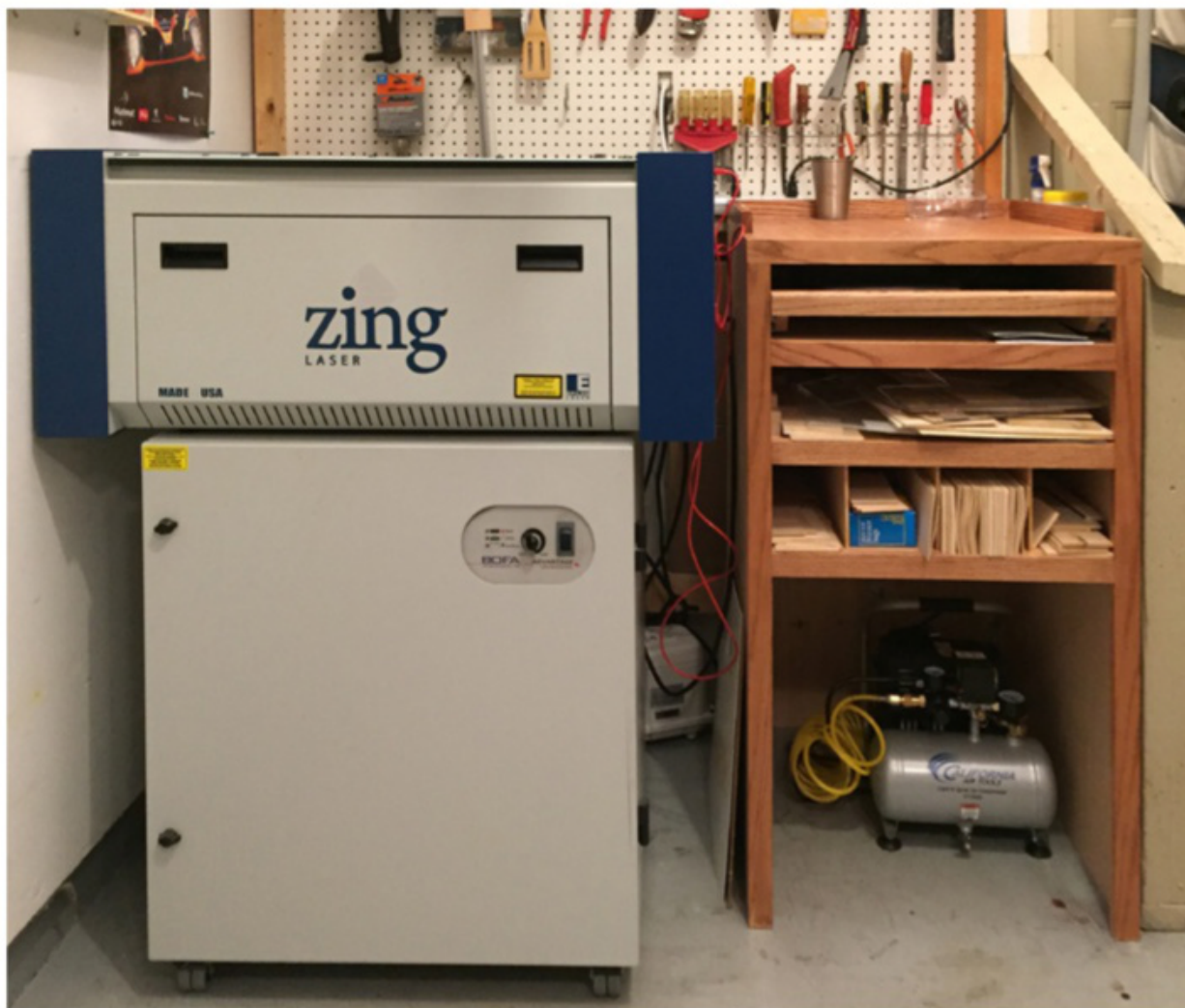
3 Laser cutter. Bernard's laser-cutting work station resides in his garage and is also used for his business, Alkem Scale Models. The Epilog Zing laser cutter has a 12 x 24-inch cutting bed and 40W of power. The laser sits on a Bofa air filter, which cleans the exhaust of smoke and toxins, a must for cutting indoors.
