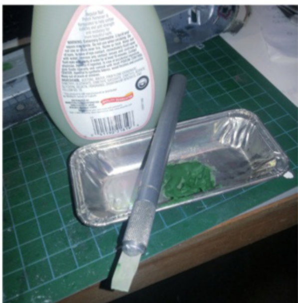
③ A little putty. Acetone makes Squadron putty easier to spread, done with a piece of plastic in a knife handle.
