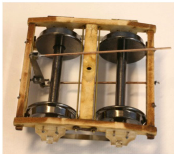
8 Working hand brakes. The truck sideframes and other main components are made of laser-cut parts. Photo-etched parts simplified constructing the working brake mechanism.
