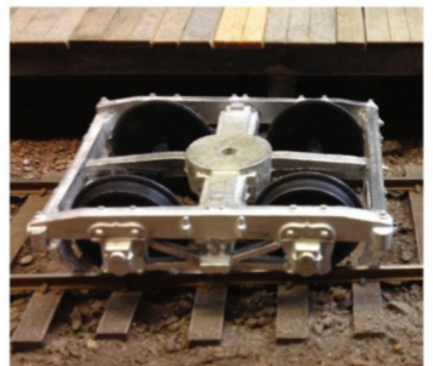
11 Spin-cast metal trucks. These metal trucks were spin cast using molds made from 3-D printed masters. The metal trucks are heavier and track better than the lighter plastic trucks.
