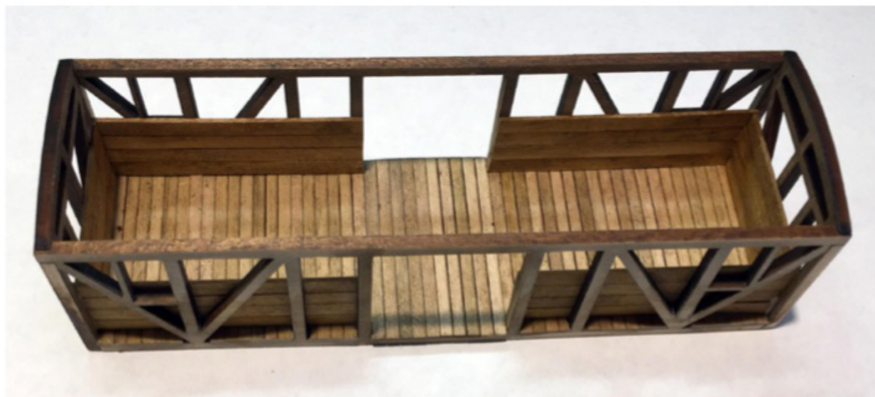
4 Freight car construction. This unfinished freight car model shows the typical method of construction Bernard uses for his laser-cut freight cars. He cuts the frame members from a single wood sheet with interlocking tabs and slots to help simplify the construction process.
