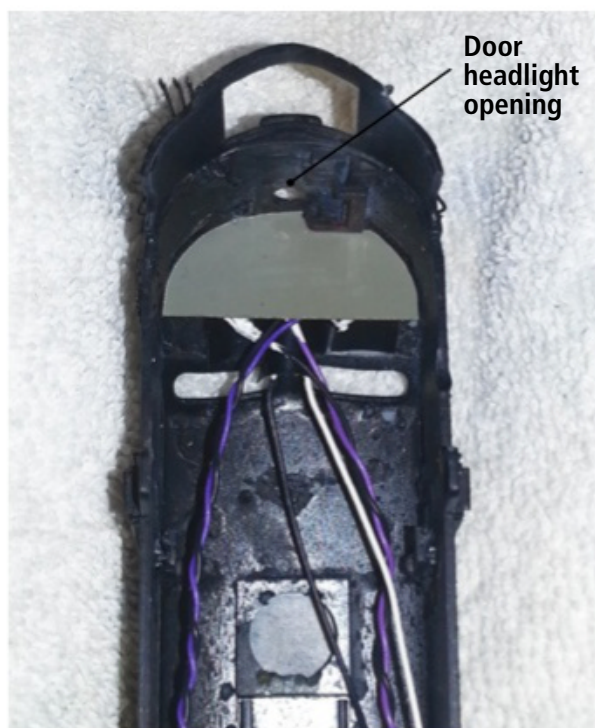
10 Mounting plate. Louis cut a styrene plate to match the curve of the inside of the locomotive shell so he could mount the next layer of lights.
