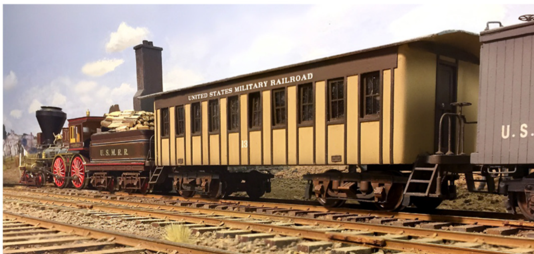
6 Finished model. Here's the finished passenger car in service on the Aquia Line. Bernard scratchbuilt the handrails from phosphor-bronze wire. The trucks are from SMR Trains.
