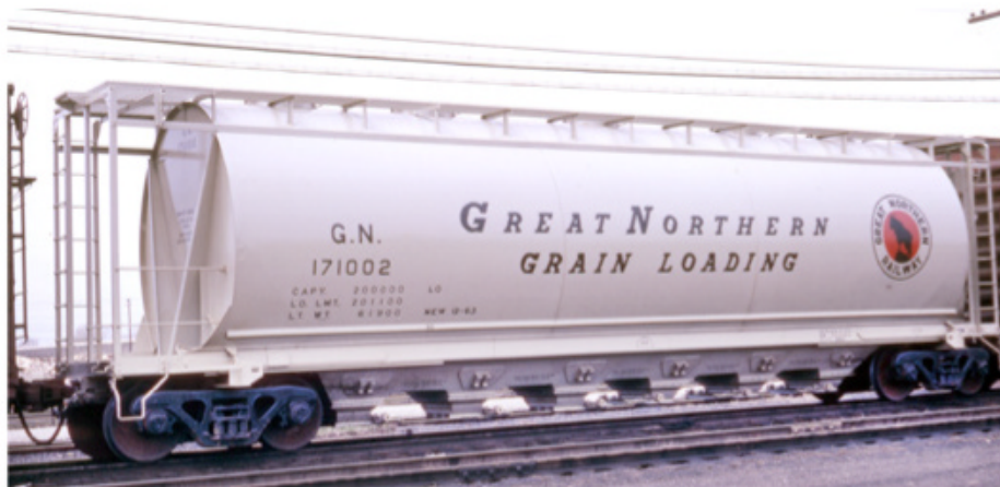
8 ACF's initial Center Flow design was cylindrical. The car has internal slope sheets, but they're covered by side and end sheathing. This 3,960-cubic-foot car was built for Great Northern in 1963. John Ingles photo; J. David Ingles collection
