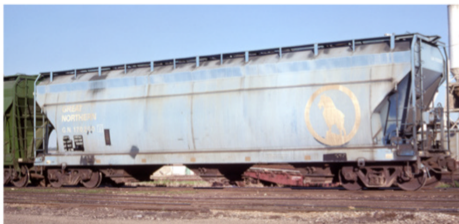
9 The teardrop-cross-section 4,650-cubic-foot car was ACF's most popular grain car. Cars built through 1970, such as this Great Northern car, have a single stiffener across the top of each side. R.J. Wilhelm photo; J. David Ingles collection
