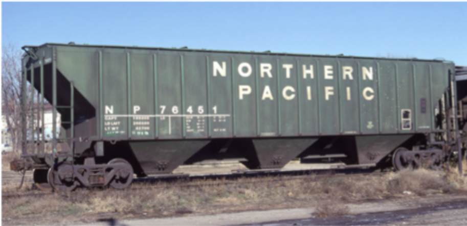
6 This 4,740-cubic-foot PS-2CD, built for Northern Pacific in 1969, has 16 evenly spaced side posts. It's almost 8 feet longer than the 4427. John Ingles photo; J. David Ingles collection
