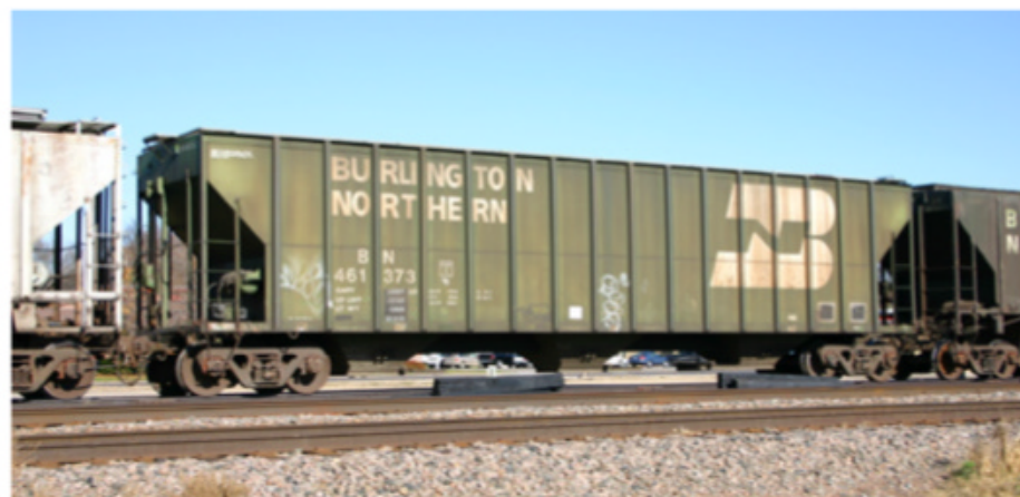
11 FMC covered hoppers have horizontal grooves running down the center of each side behind the posts. The 16 side posts mark this Burlington Northern car as a 4,700-cubic-foot version. Jeff Wilson photo
