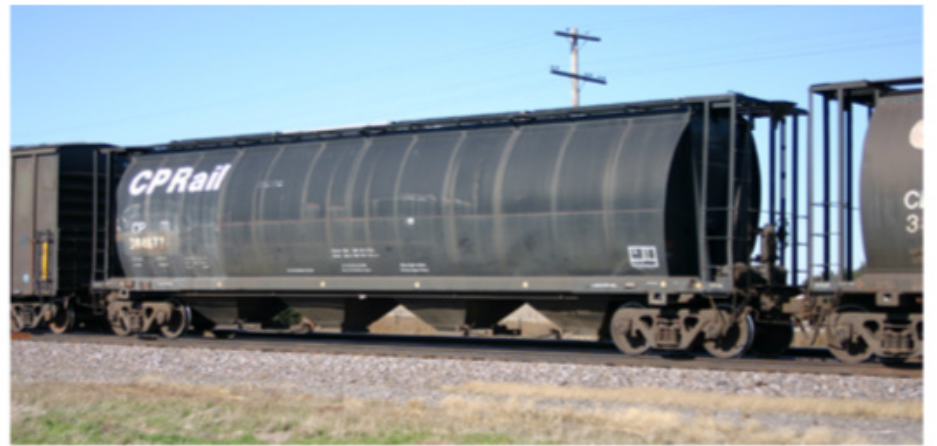
14 Canadian railroads acquired large fleets of cylindrical covered hoppers, built to common designs by three manufacturers. This Canadian Pacific car has a 4,550-cubic-foot capacity. Jeff Wilson photo
