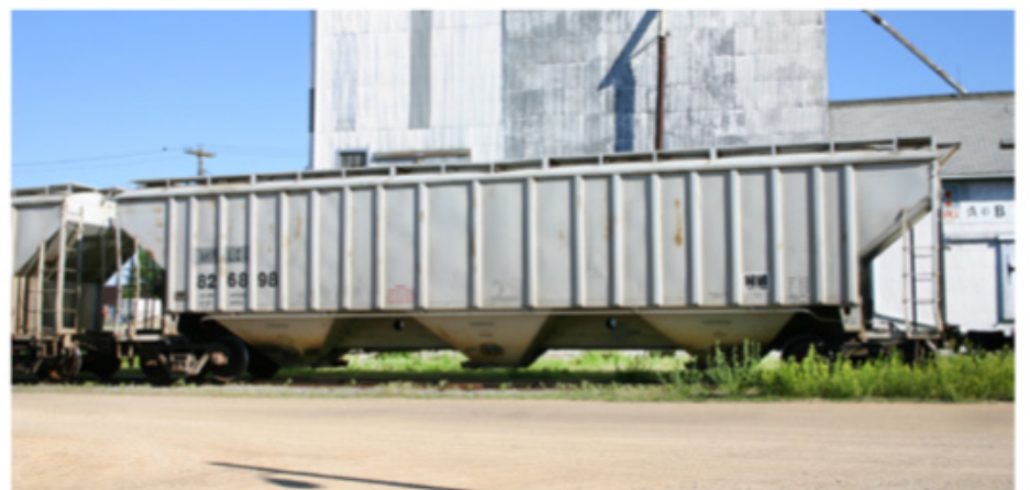
15 This 4,750-cubic-foot car was built by Richmond Tank Car, and can be spotted by its 19 unevenly spaced posts. Originally built for North American's lease fleet, it's now owned by Minnesota Prairie Line. Jeff Wilson photo
