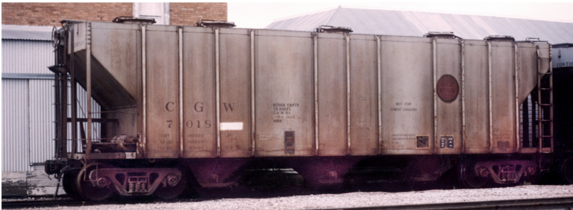
③ Pullman-Standard's first true grain car was the 4,000-cubic-foot, three-bay PS-2CD. The design was introduced in 1962; this Chicago Great Western car, built in 1963, has round roof hatches that would soon be rare on grain cars. Jeff Wilson collection
