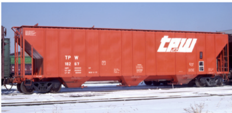
13 Evans built this 4,780-cubic-foot car for Toledo, Peoria & Western in 1977. These cars have a 5-4-5 post pattern and tall sides. You can see the edges of the corrugated roof panels.
