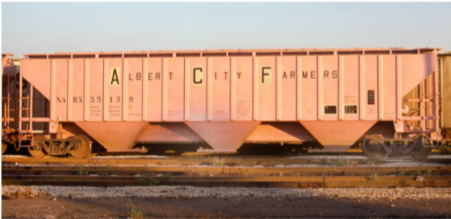
7 The 4,750-cubic-foot hopper was Pullman-Standard's most-popular grain car, and many are still running. Built for North American's leasing fleet in 1974, this one is painted for an individual elevator. R.J. Wilhelm photo; J. David Ingles collection
