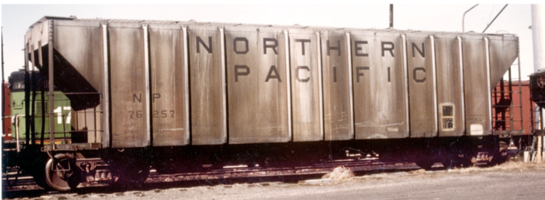
④ The 4,427-cubic-foot PS-2CD is noticeably longer than the 4000. Early versions share the same deep sides and 4-3-4 post pattern. This Northern Pacific car was built in 1966. Jeff Wilson collection
