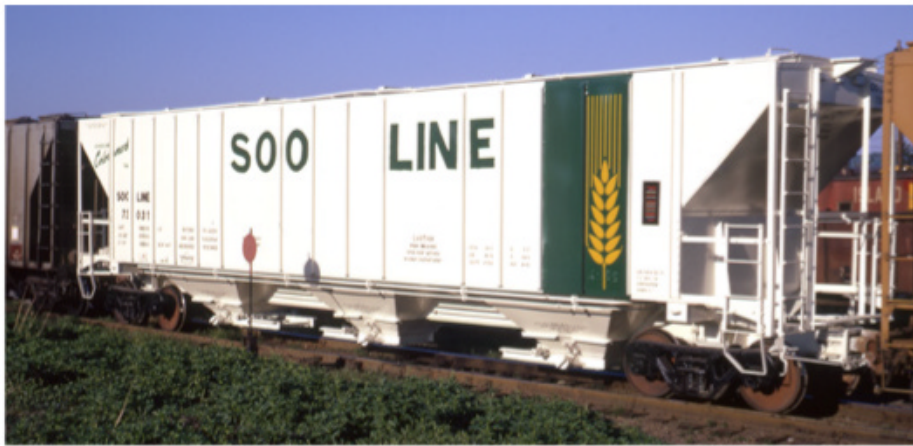
12 Thrall built this 4,750-cubic-foot car for Soo Line in 1971. It has combination gravity-pneumatic outlets, a 6-4-6 post pattern, and the verticals at each end are actually U-channels.
