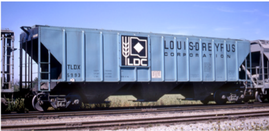
5 Late versions of the 4427 had 13 side posts and shallower sides. This car, part of the Pullman Leasing fleet, was built in December 1966 and lettered for lessor Louis-Dreyfus. John Ingles photo; J. David Ingles collection
