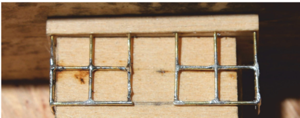
6 Railing. The railing was bent and soldered together using brass wire, then mounted to holes drilled in the end platforms.
