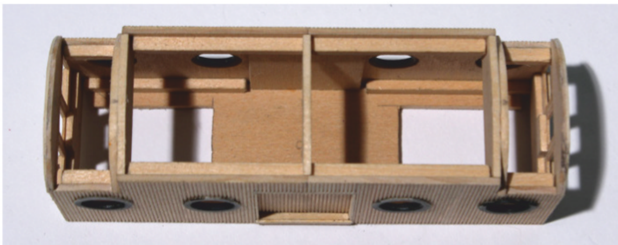
5 Framing it up. The sides and ends have been assembled into a single unit, with the roof bracing installed.
