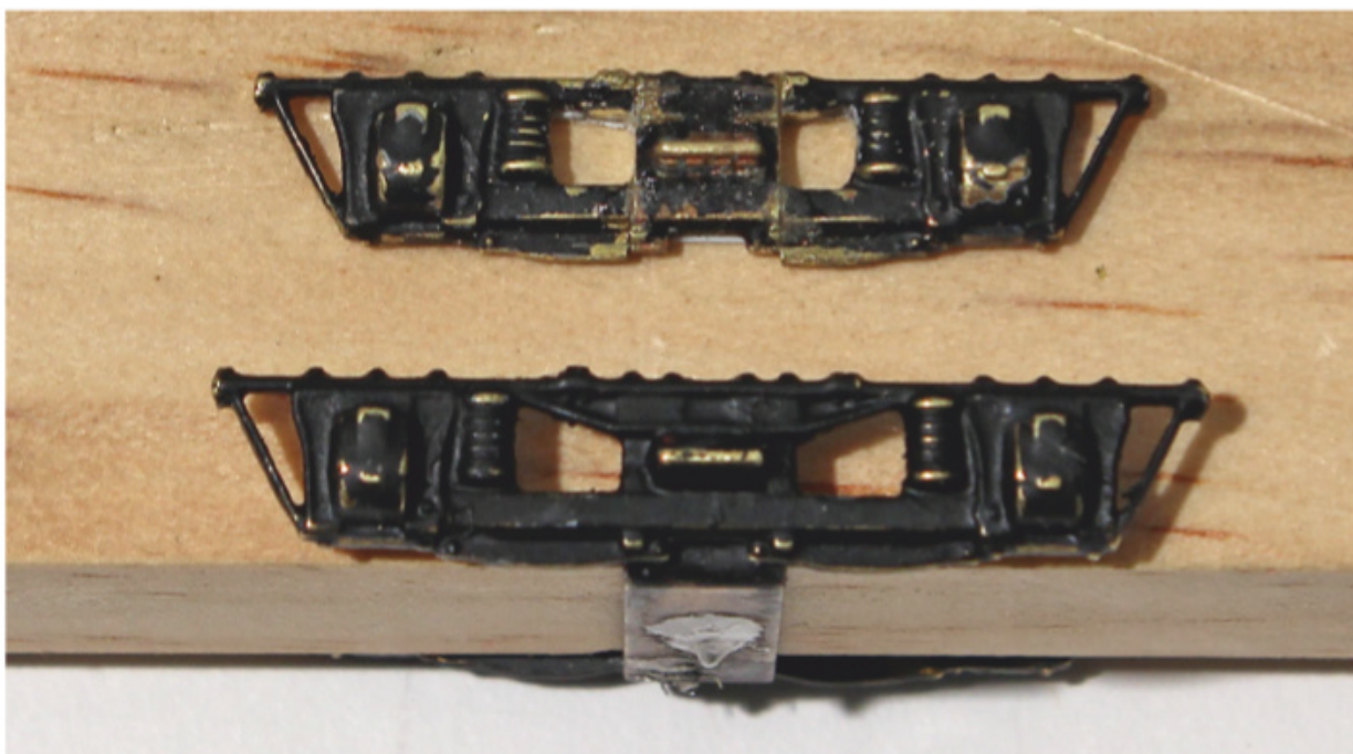
8 Shorter side frames. The donated side frames have been shortened to match the dimensions of the power trucks. The original-length truck is on the bottom.
