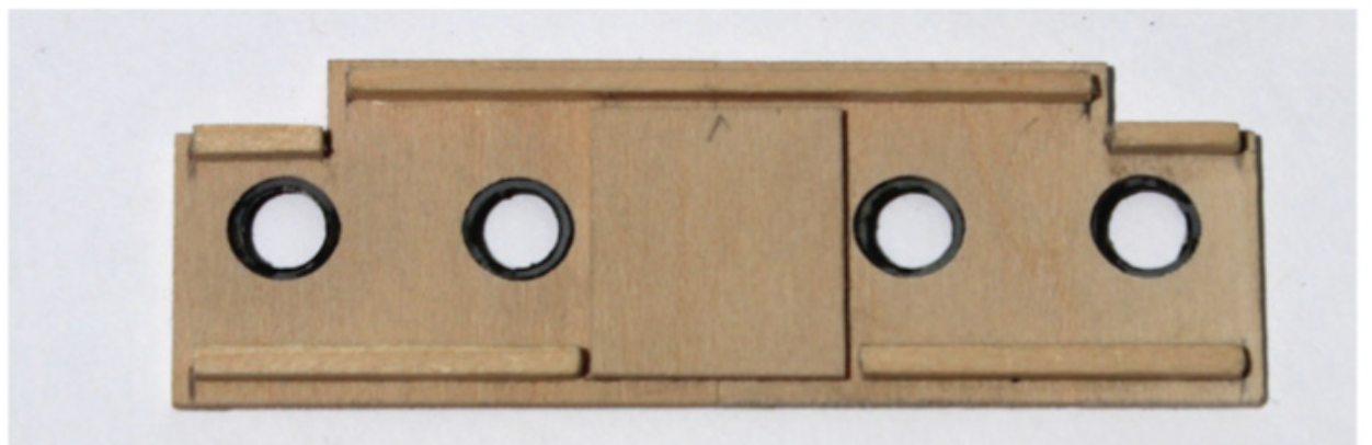
③ Bracing. Stripwood bracing has been applied to the back of the side, with sufficient room at the bottom for the floor.
