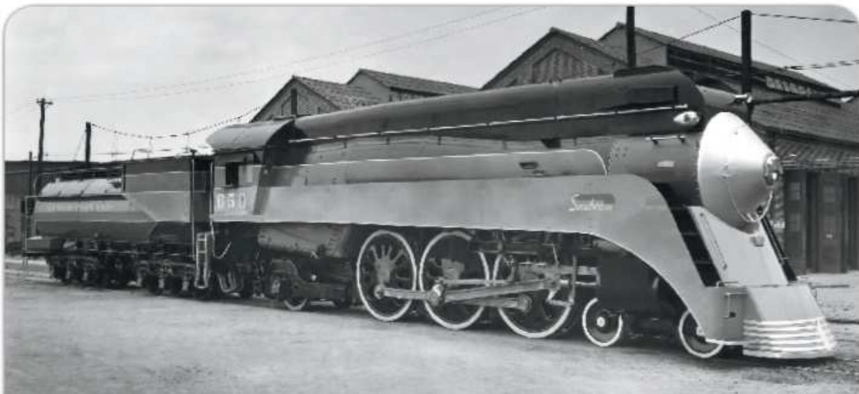
Southern Pacific 4-6-2 Pacific no. 650 is resplendent in Daylight livery as it stands ready to pull the crack passenger liner Sunbeam between Houston and Dallas. Like many SP steam locomotives, no. 650 is fed by a cylindrical Vanderbilt tender, seen behind the cab. Southern Pacific photo
