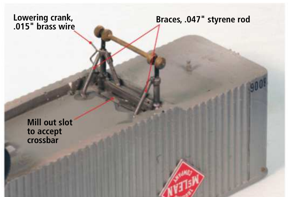
Trailer landing gear comes in two heights: retracted, for towing; and lowered, for standing alone.
