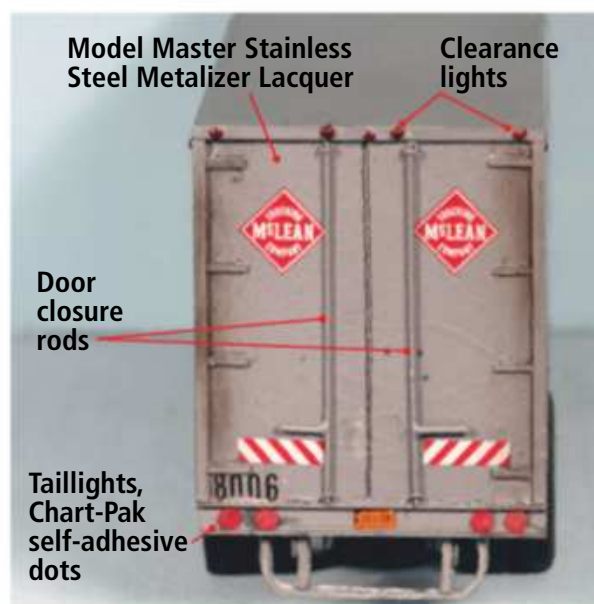
The clearance lights are the heads of small brass nails, painted red.
