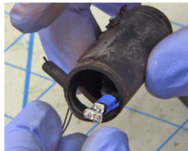
To install the Evan Designs fire kit, I taped the 3 LEDs together and placed them inside the boiler pointing down into the firebox.
