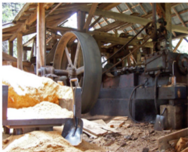
Phillips Brothers main steam plant sits near the boiler, which is just out of the picture to the left. The sawdust is used to feed the firebox. G. Hendrix photo
