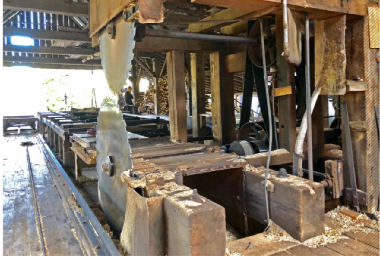
The Phillips Brothers mill uses a saw with two blades to handle the bigger logs. The lower blade makes most of the cuts. The upper blade is activated only when needed. G. Hendrix photo
