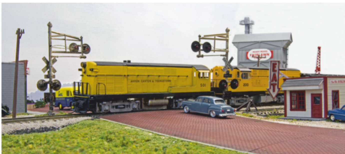
8 Fairbanks-Morse H20-44 no. 501 leads H15-44 no. 200 across brick-paved West Market Street in Akron, Ohio, with westbound freight No. 95. The Beloit, Wis.-built diesels featured opposed-piston diesel engines.
