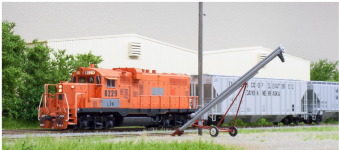
5 Lake Valley & Northern's "newest" motive power is a well-worn GP10 rebuild from Illinois Central's Paducah, Ky., shops. Locomotive no. 8229 is an InterMountain model with Detail Associates wipers, Cannon & Co. radiator fans, an ESU LokSound decoder, and a "patched out" paint scheme.
