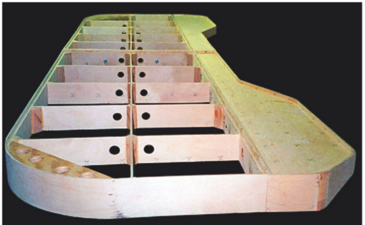
George Nefstead built the strong yet lightweight benchwork in two mirror-image halves from thin birch plywood. The "indented" area at the right of the display layout is planned as the site of a future staging yard.
