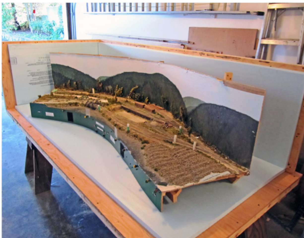
The second smallest section, Bear Creek, was over 200 pounds once crated. Here it sits secured to the crate base. The foam insulation was added at the request of the museum to help avoid thermal shock. Mark Dance photo
