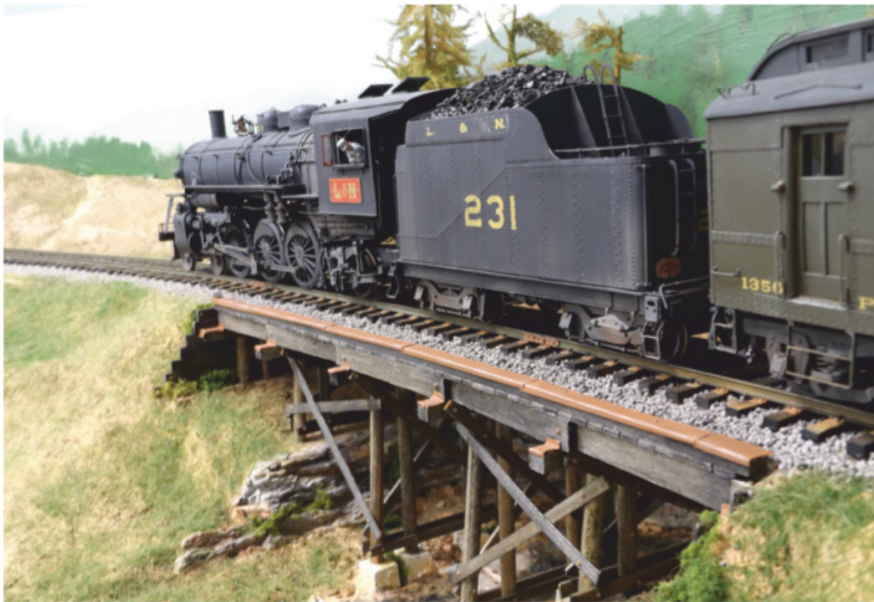
3 The fireman takes a look at the train as Pacific no. 231 rounds a curve to the left while crossing bridge 80, a ballasted-deck timber trestle over Dry Creek. Note the metal rain-and-hot-cinder guards atop the stringers.
