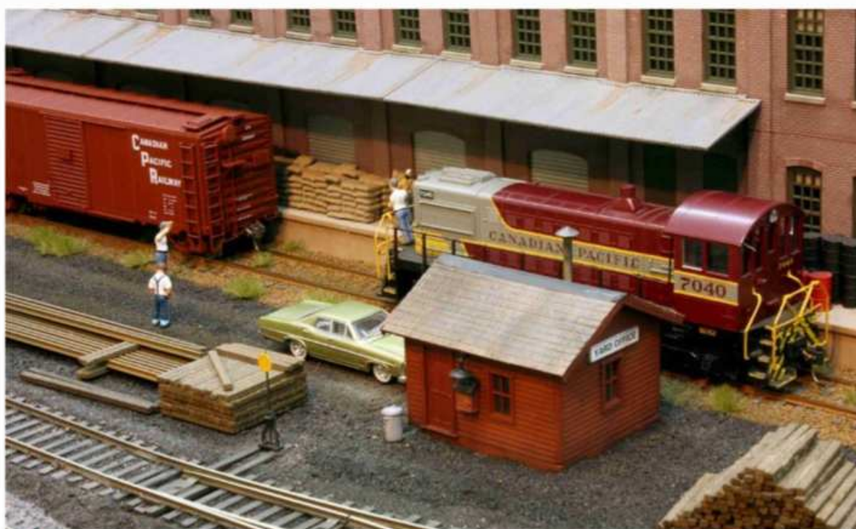
5 CP 7040, an Alco S-2, switches General Foods in LaSalle. Ian achieves the slow speeds needed for realistic switching by keeping his track and wheels clean, rostering free-rolling and properly weighted cars, and using high-quality walkaround throttles.
