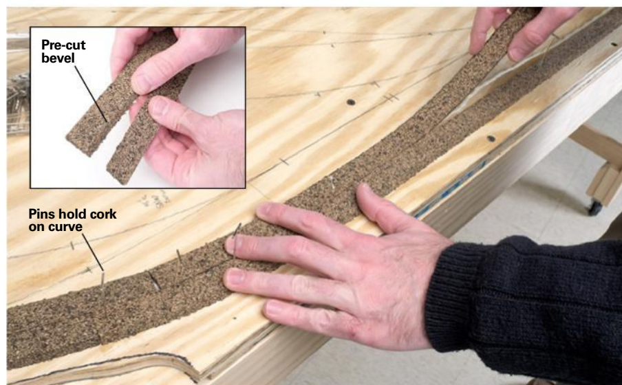
Fig. 1 Laying cork strips. Midwest cork is split down the middle (inset photo). Separating the cork into two pieces makes it easy to lay it on curves (above).
