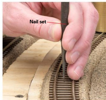
Fig. 5 Track nails. Once a section of track was positioned, David tacked it with track nails so it wouldn't move while he worked on the next section.
