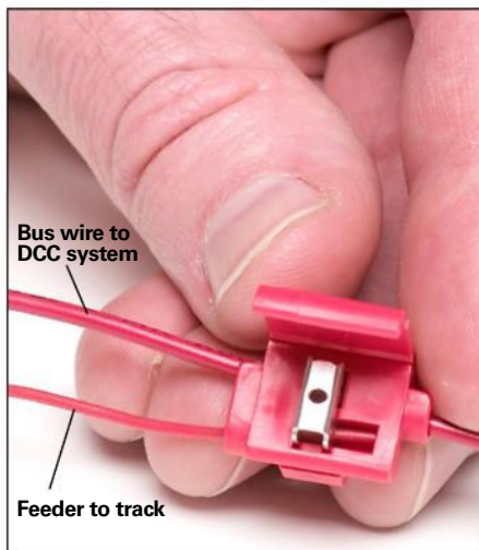
Fig. 9 Power bus. David used 16AWG wire for the power bus under the layout, connecting the smaller feeder wires to insulation displacement connectors (suitcase connectors).
