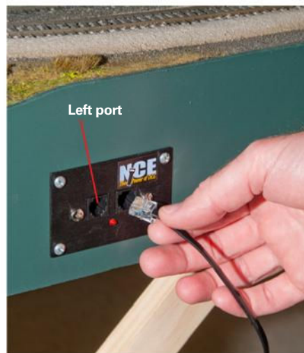
Fig. 12 PowerCab connection. The PowerCab is the brains of the system and must remain plugged into the left socket of the main cab bus port (the one with the red LED) at all times.
