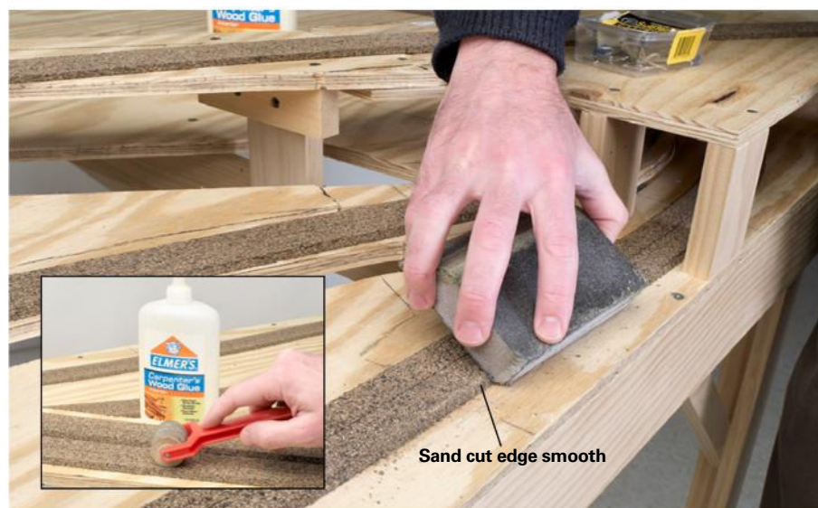
Fig. 2 Smooth on all sides. With the cork set in the glue, David smoothed it with a wallpaper roller (inset). After the glue dried, he sanded the cut edges.
