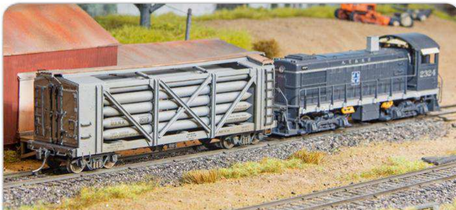
Helium cars, like this HO scale Ambroid model built by Model Railroader associate editor Eric White, were made of an array of horizontal high-pressure tanks, each of which was loaded and unloaded separately. Bill Zuback photo
