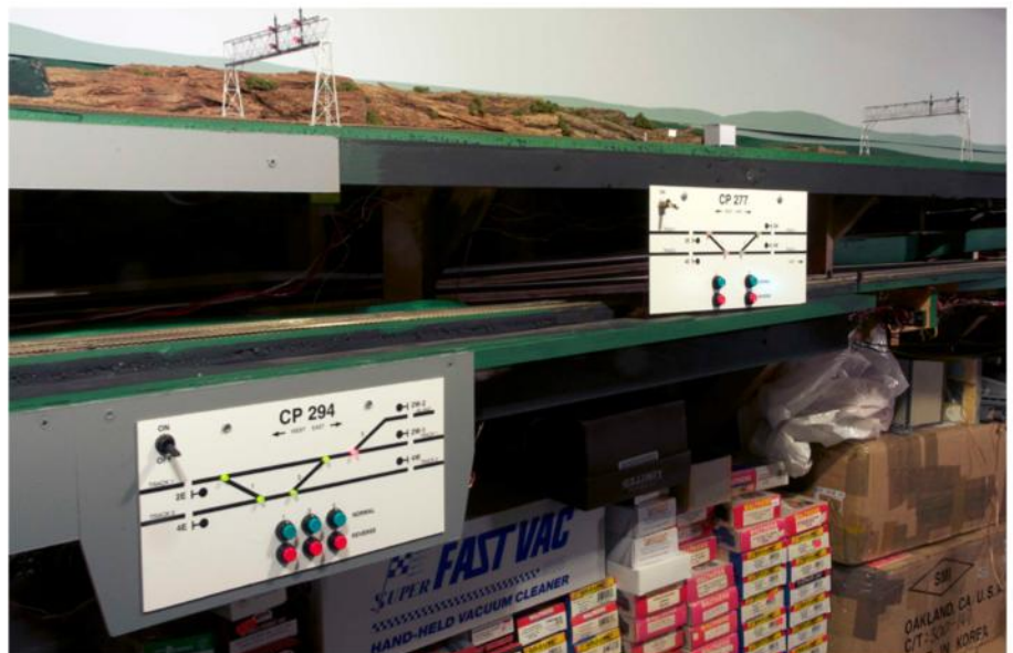
9 Panels along the fascia provide location labels as well as local control for crossovers, here at Control Points 294 and 277. The on/off switches help ensure the crossovers are lined with dispatcher permission, even when on local control.
