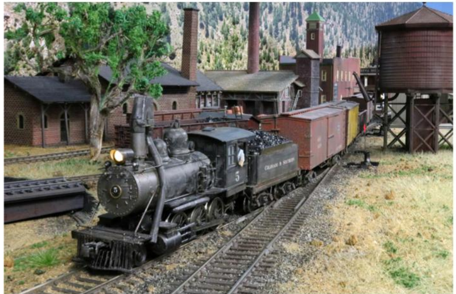
5 C&S engine no. 5 pulls a short freight out of Idaho Springs on its way to Denver. Doug made this 2-6-0 engine by shortening the frame and removing the second driver of an Athearn/Roundhouse 2-8-0 locomotive.
