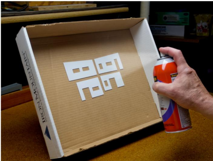
❷ Several quick passes of spray adhesive over the styrene walls and voilà – a textured finish that's easy to see and looks like the real thing. The copier paper box lid helps catch the sticky overspray.
