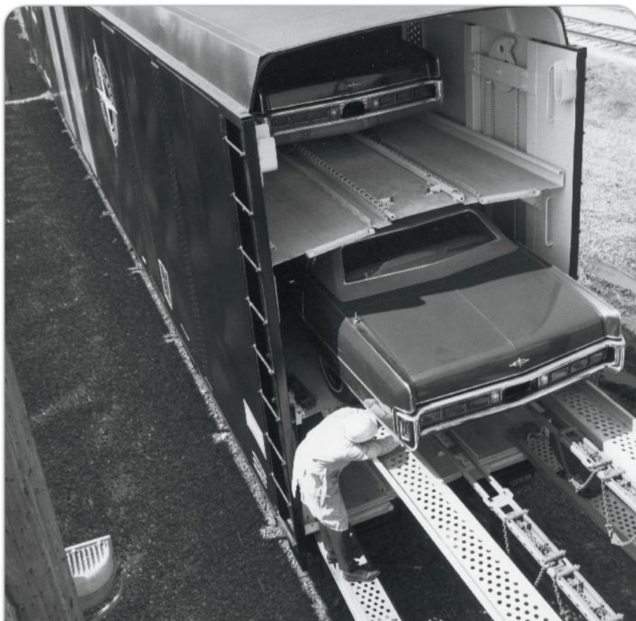
A worker adjusts the automatic tie-down mechanism on a new 1973 Lincoln Continental as it's loaded into a Detroit, Toledo & Ironton enclosed auto rack car at Lincoln's assembly plant in Wixom, Mich. Note the cars are loaded to one side to let the drivers out. Ford Motor Co. photo
