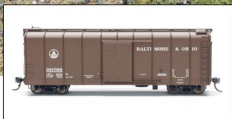
This HO scale Baltimore & Ohio class M-15k boxcar is modeled as the prototype appeared in 1946. The basis of the model is a Fox Valley Models class M-53 boxcar (inset) with modified sills that rides on an Accurail fish-belly frame. Bill Zuback photos
