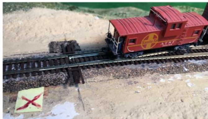
X marks the spot where the switch rod used to be. After several years of sporadic derailments at this turnout, Jim Kelly relocated it a few inches from the curve so engines would get a short straight before entering the turnout. Roen Kelly photo
