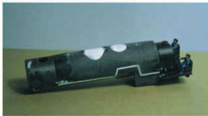
Fig. 4 STRIPPED BOILER. The only details that Iain left on the boiler are the smoke-box rivets.
