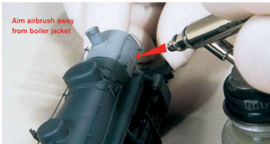
Fig. 4 When painting the smokebox, John aims the nozzle of the airbrush forward and away from the boiler (the boiler actually begins at the rear of the smokebox). With a little practice, even small areas of different color can be painted by careful aiming.
