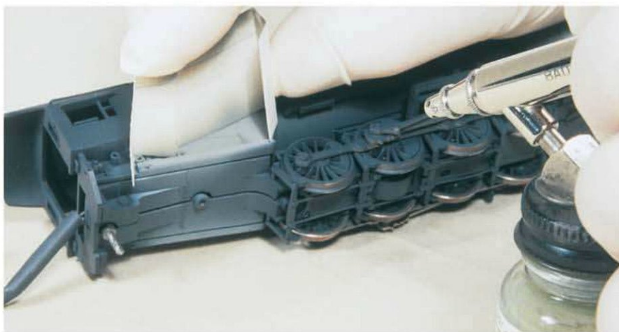
Fig. 5 John uses baffles to mask adjacent colors. This baffle was cut from an index card and bent to the shape of the firebox. John holds it in place while the firebox is being sprayed ash gray to protect the Grimy Black cab, drivers, and running board.
