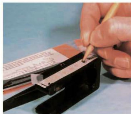
The lettering is burnished onto the surface of the model using an HB pencil. David makes sure he covers all the letters completely.
