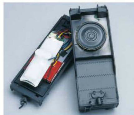
Fig. 15 TENDER. The shortened tender still has enough room for the Bachmann circuit board. No. 472 was equipped with a SoundTraxx steam sound decoder and a speaker and put to work on the layout.
