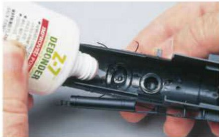
Fig. 2 UNSTICKING DOMES. Apply some CA debonder to the inside of the domes and stack and let it sit for a few minutes.
