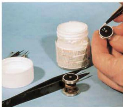
David uses a ruling pen and paint to stripe the tires. The trick is loading enough paint to complete the tire without stopping.
