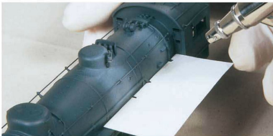
Fig. 6 Another use of a baffle is to prevent the ash gray paint streaks on the boiler from getting on the Grimy Black running boards. This baffle fits snugly against the boiler on top of the running board, and John cut notches to clear cast-on piping.
