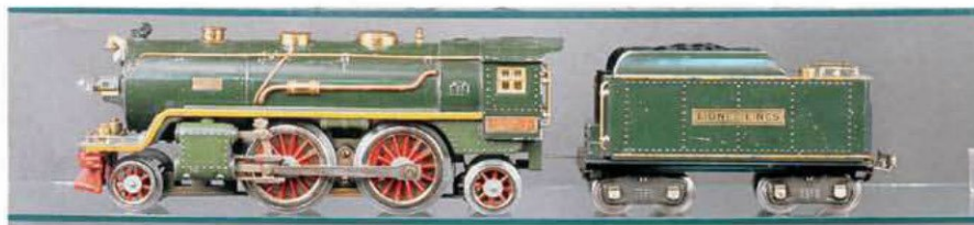
Fig. 1 The Lionel 390E of 1929 was typical of early tinplate steam engines. It had many compromises in proportions and details, and its shiny paint, brass domes, and a bulb sticking out of the headlight made it look more like a toy than a prototype locomotive.
