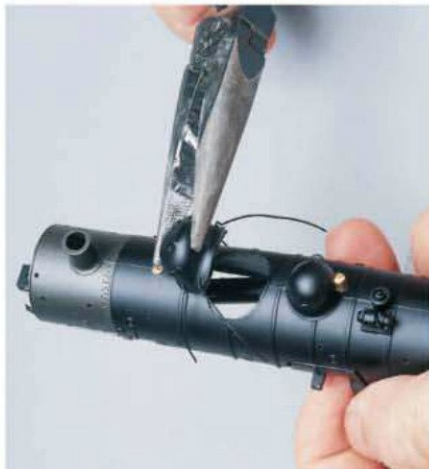
Fig. 3 REMOVING DOMES. Then use pliers to grasp the domes. They should easily lift right off the boiler.
