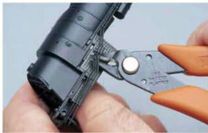
Fig. 1 REMOVING PIPES. Use flush-cutting nippers to remove the plastic pipes from the boiler. Leave the mounting pins in place.
