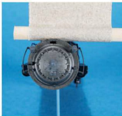
Fig. 10 SANDER. John uses a dowel covered with sandpaper to create a slot for a feedwater heater tank.
