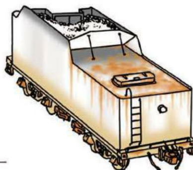
Fig. 2 TYPICAL TENDER WEATHERING PATTERN
