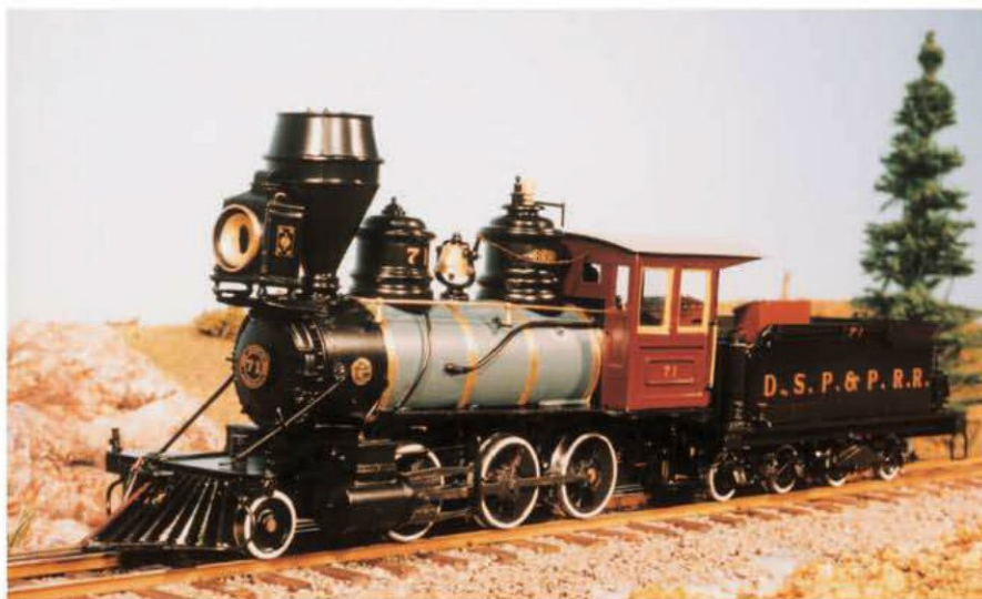
The Denver, South Park & Pacific's Moguls were certainly colorful locomotives. Here David Steer describes how he painted this Sn3 brass model of no. 71.
