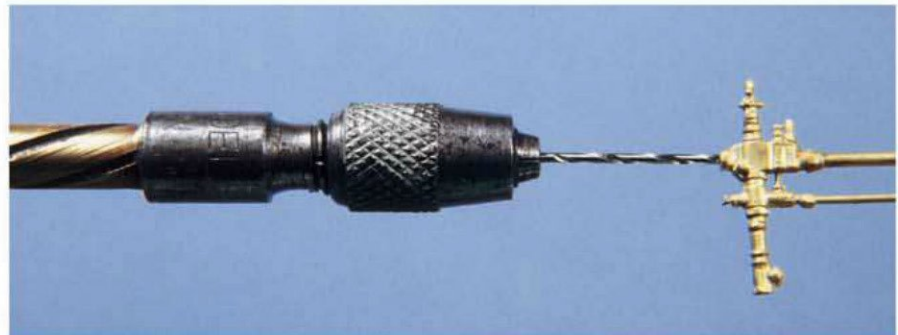
Fig. 6 PIPE HOLE. Using a pin vise and a bit .002"- .003" larger than the pipe, John drills a hole for a pipe \frac{1}{32} " deep in a lifting injector casting.
