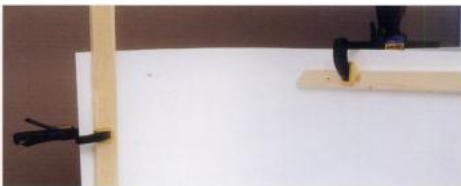
Secure the styrene backdrop to the frame with water-based contact cement and clamp it in place.
