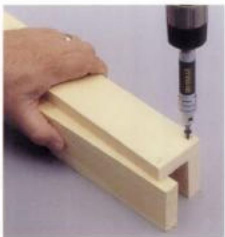
Lionel used a countersink tool to countersink the pilot holes for the screws. Here he's assembling the L girders.
