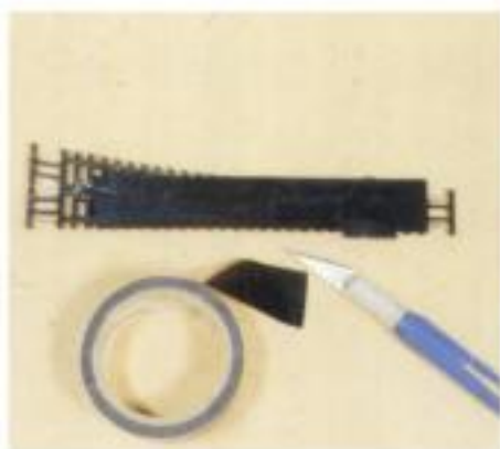
Fig. 2 PREPARING TURNOUTS. Add electrical tape to the back of each turnout, covering the throw rod as well as the ties out past the frog.
