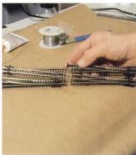
Fig. 1 SOLDERING TRACK. Solder turnout groups together before adding them to the layout. Use rosin flux (shown here in a tube and applied with a brush) to help the solder flow into the rail joints.
