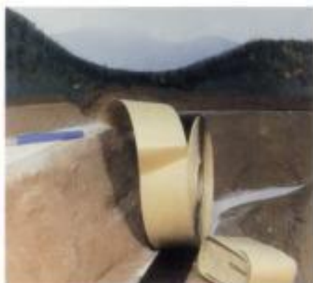
Fig. 3 LAYING ROADBED. Roll the AMI Instant Roadbed along the track center line. A wood block covered with waxed paper works well for pressing the roadbed into place.
