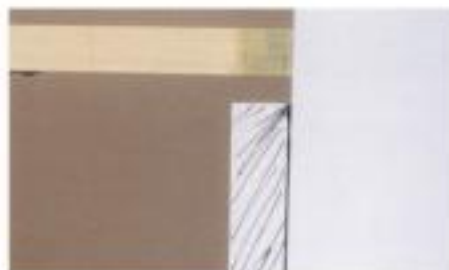
To join two pieces of styrene Lionel cut a splice plate from scrap material and secured the pieces together with cyanoacrylate adhesive (CA).
