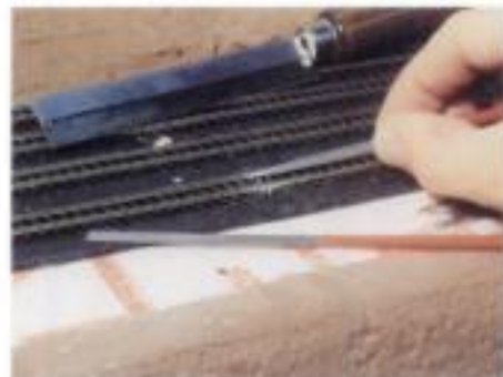
Fig. 2 RAIL GAPS. Cut the rail gaps with a razor saw, then glue small pieces of .010" styrene into the gaps to ensure that the rail ends stay apart. Trim the styrene to shape with a hobby knife and files.
