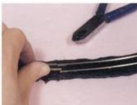
Fig. 4 TRIMMING FLEXTRACK. When bending flextrack the ends won't come out even. Use a rail nipper to trim the longer rail to length, then use a small file to make sure the end is square. When the fit is good, set the track in place with rail joiners and solder the joints.
