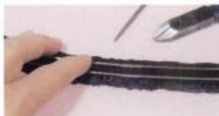
Fig. 4 TRIMMING FLEXTRACK. When bending flextrack the ends won't come out even. Use a rail nipper to trim the longer rail to length, then use a small file to make sure the end is square. When the fit is good, set the track in place with rail joiners and solder the joints.
