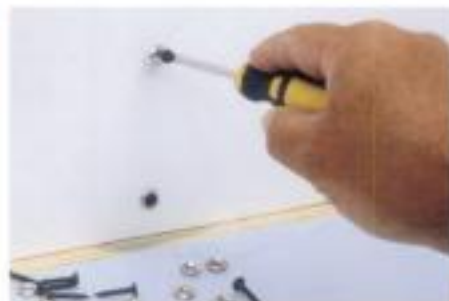
In areas that will be hidden by scenery use drywall screws to attach the backdrop to the frame.
