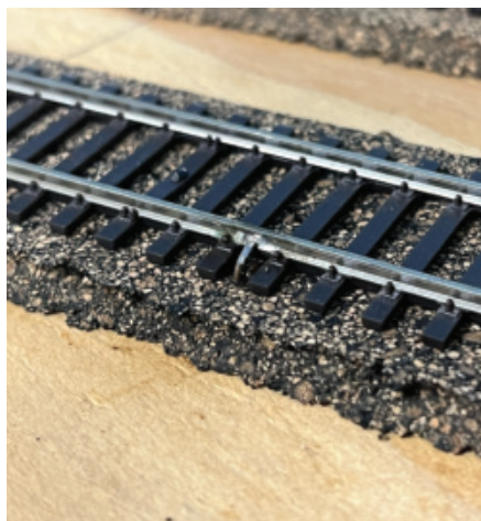
After stripping ¼" of the insulation from the feeder, the staff soldered it to the web of the rail, as shown here.
