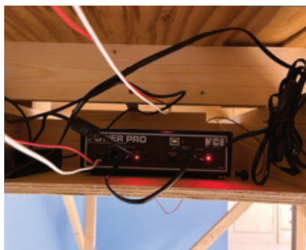
We used a piece of plywood to make a shelf under the layout to hold the DCC system and power supply.
