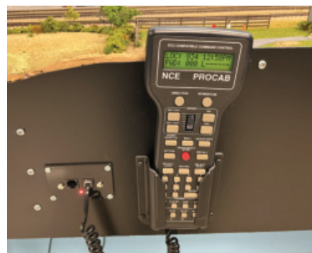
We mounted Universal Throttle Pockets from PPW-Aline.com on the fascia next to the plug ports to hold the cabs.
