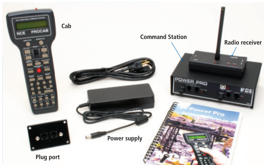
For our East Troy layout, we chose an NCE PH5-R wireless Power Pro Digital Command Control system. This set is easily expandable as your layout gets bigger.
