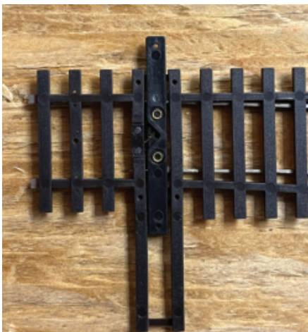
To use Walther's turnouts with its switch machines, you must first remove the toggle spring, attached between the left headblock tie and the switch rod.
