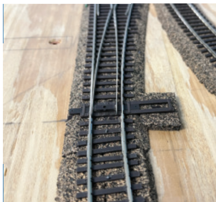
Whether using strips or pads for turnouts, be sure to include a tab to support the headblock ties.
