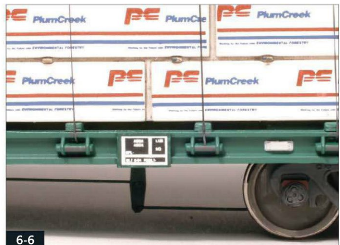
Fix a stencil decal to a styrene sheet and glue it to the side sill of a flatcar.
