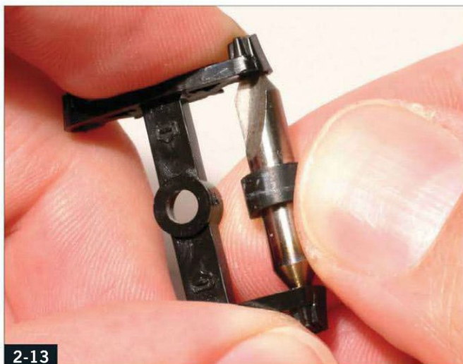
2-13 Micro-Mark's Truck Tuner reams out the needlepoint pockets on HO truck sideframes, removing flash and improving operation.
