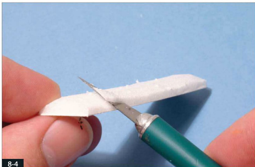
Foam is easy to carve into shaped bases for coal and other bulk loads.
