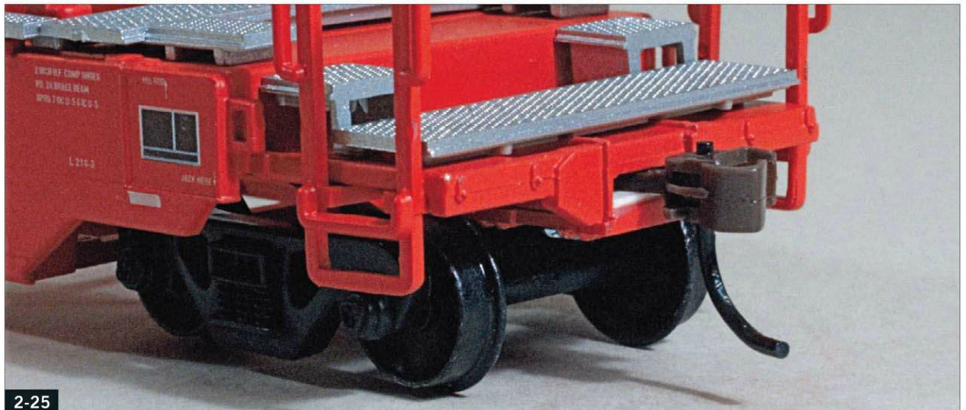
2-25 The coupler is now level – and the uncoupling pin has been fixed as well.
