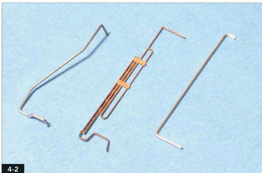
4-2 Available uncoupling levers in HO include DA no. 6215, Plano no. 12002, and DA no. 6240.
