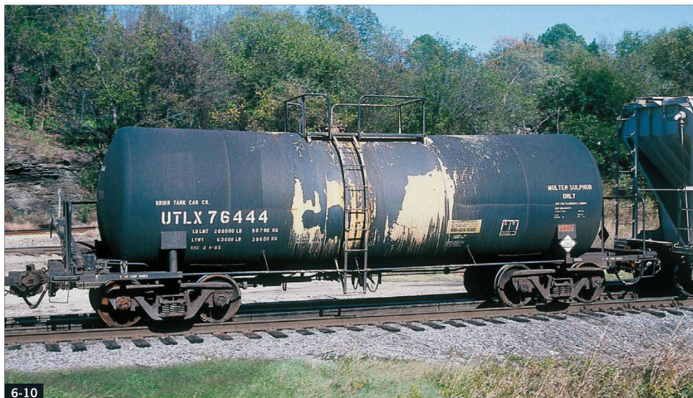
This tank car is placarded for molten-sulfur service, with the commodity stenciled on the side, orange decals with the commodity number, and diamond-shaped placards.
