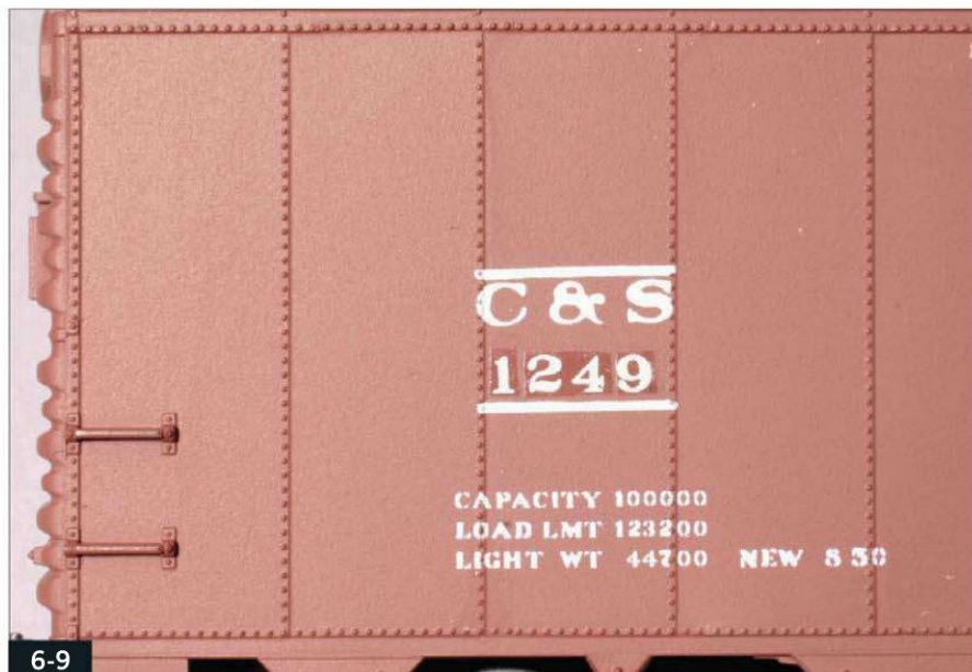
Use decals from a matching set to add the new road number.
