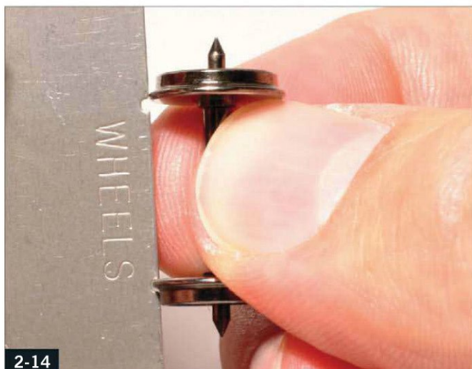
2-14 The wheel flanges should fit in the "wheel" slots on an NMRA standards gauge. This wheelset is wide in gauge.
