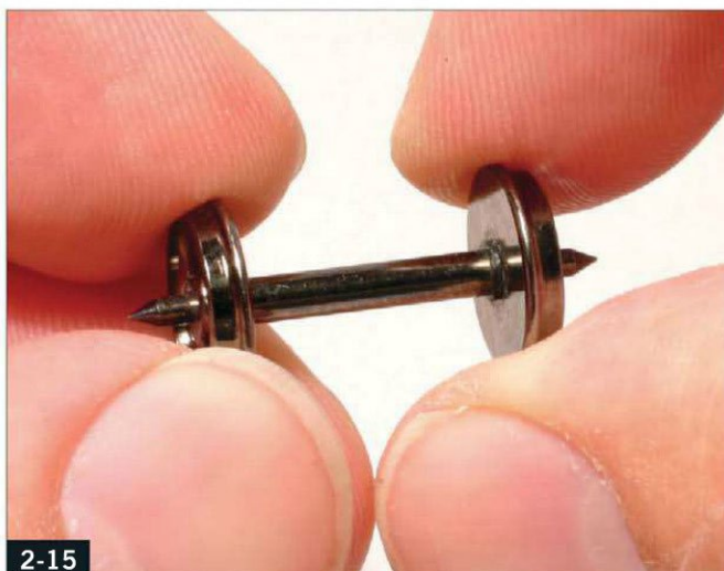
2-15 To adjust the gauge, grab both wheels firmly and twist while pulling or pushing them on the axle.
