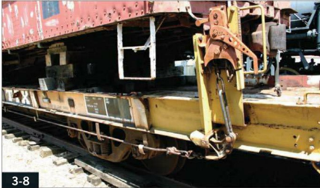
3-8 The rod from the brake lever to the cylinder is exposed along the side of long piggyback flatcars.
