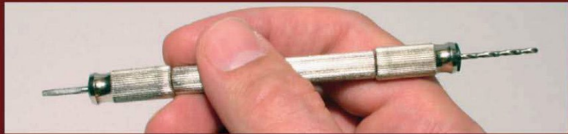
This double-ended pin vise from Mascot keeps a matching tap and drill together.
