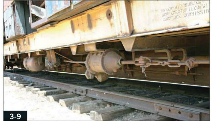
3-9 The cylinder, valve, and reservoir are prominent, as they hang below the side sill.
