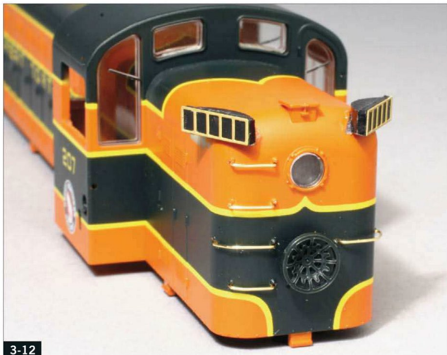
3-12 Glue the etched-brass frames to the faces of the number boards. This view also shows the grab irons in place.
