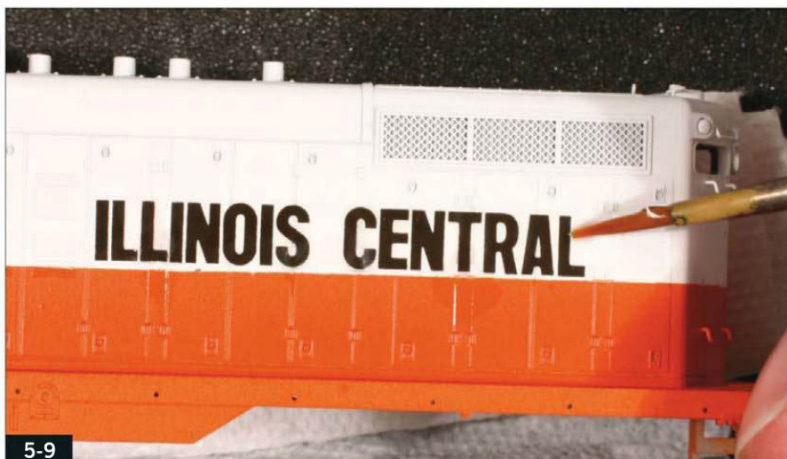
Use a soft brush to nudge the decal into position. Apply decal setting solution around the edges, being careful not to move the decal.
