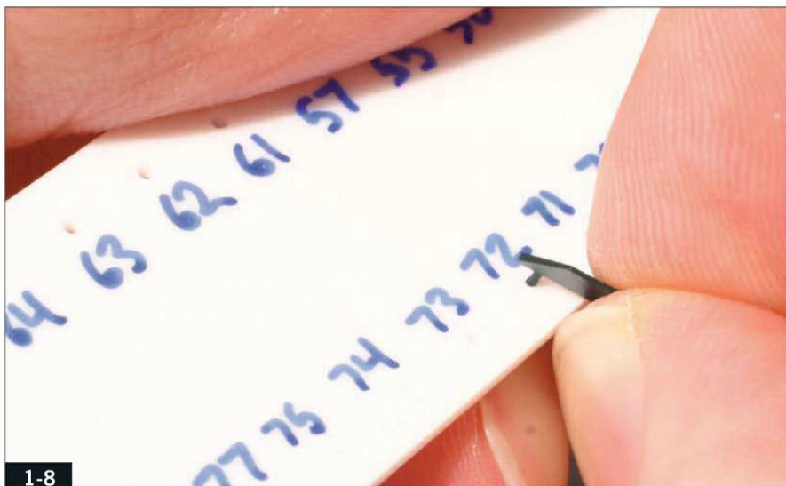
1-8 Make a drill bit template by drilling holes around the edge of a thick piece of styrene. This cab sunshade will need a No. 72 mounting hole.
