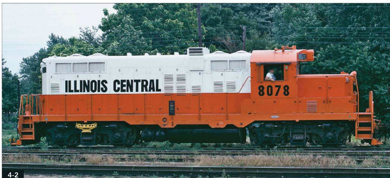
Illinois Central GP10 No. 8078 was just two months out of the shop when this photo was taken in June 1970. Note the lack of snow hoods on the air filter atop the hood. John Ingles; J. David Ingles collection
