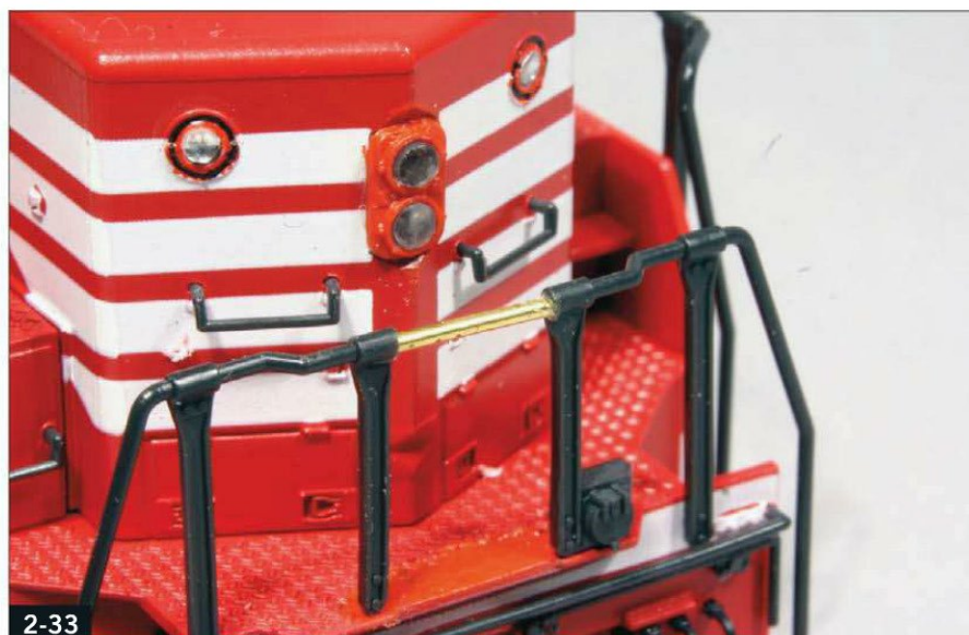
The new handrail blends with the original. Paint it black to match.
