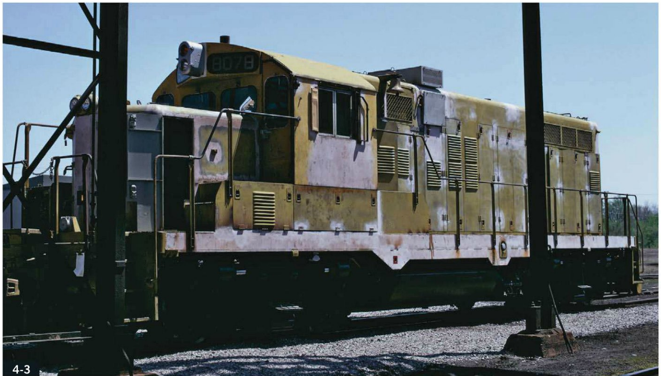
This view shows No. 8078 during rebuilding in April 1970, before passing through the paint shop. The notched access door on the side of the nose is standing open. John Ingles; J. David Ingles collection
