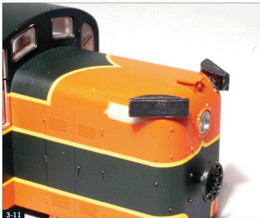
Glue the number boards in place at a 45-degree angle. Fill any gaps at the rear with CA.
