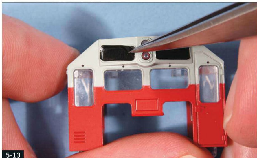
5-13 Apply the number board background first, then let it dry completely before adding the numerals.
