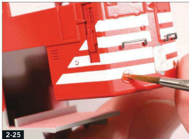
2-25 Paint out the white stripe with body color inside the class-light casting.
