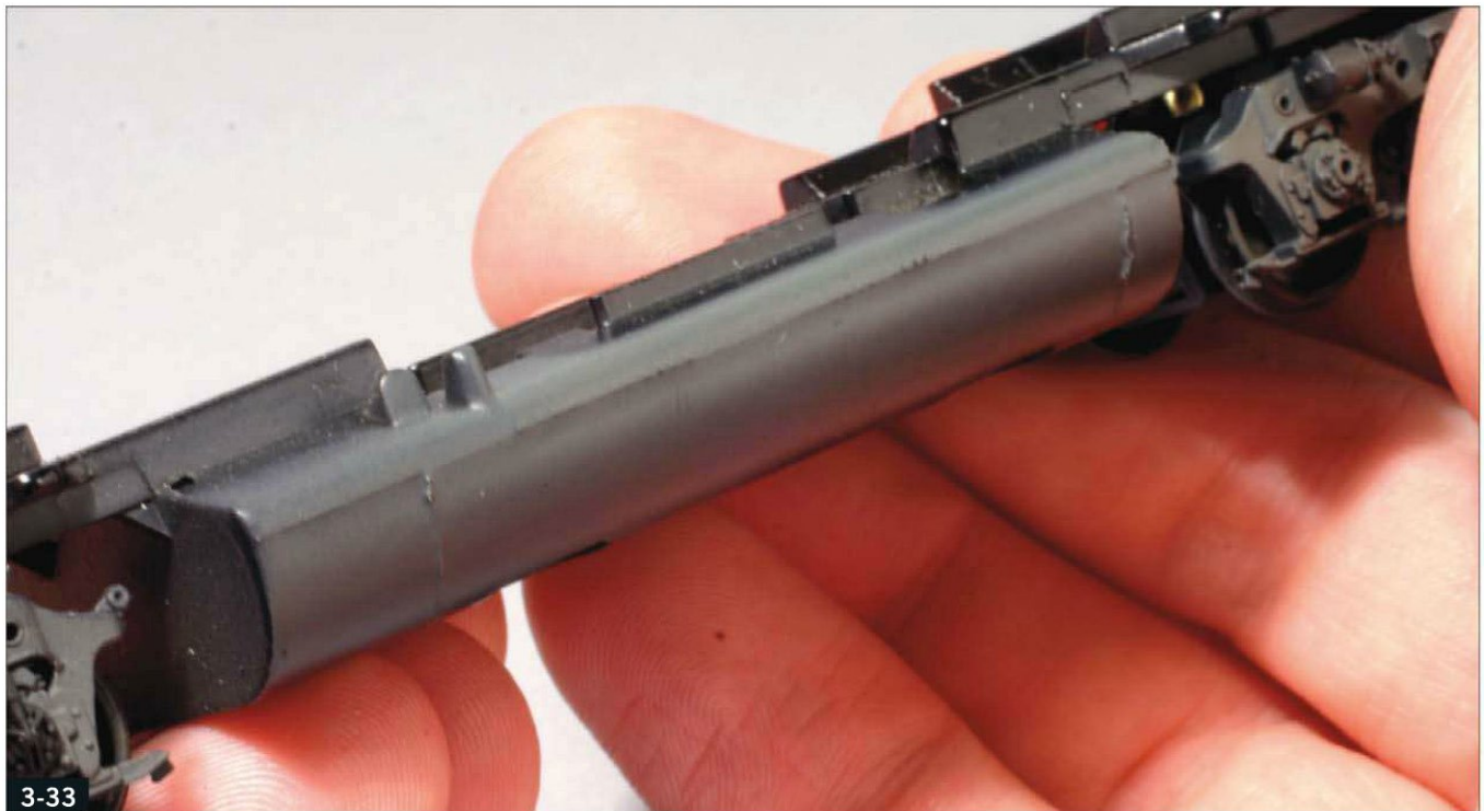
The metal Athearn chassis has a molding line and other imperfections across the fuel tank, and the filler and sight glass details are crude.
