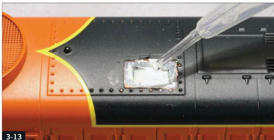
3-13 Add a few drops of CA to the opening, then use a pipette to add CA accelerator. Repeat the process until the gap is filled.
