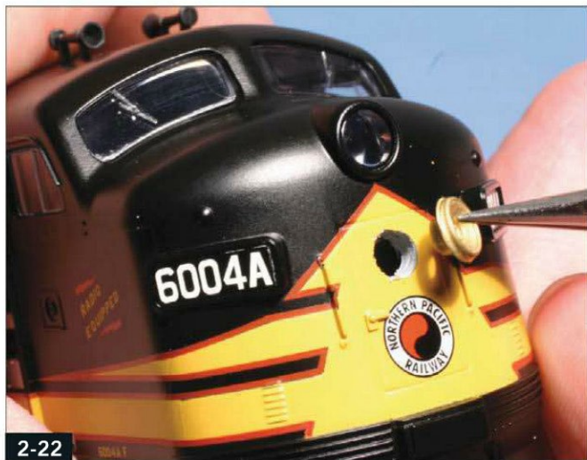
2-22 Test-fit the new lower headlight in its mounting hole, then glue it in place with CA.
