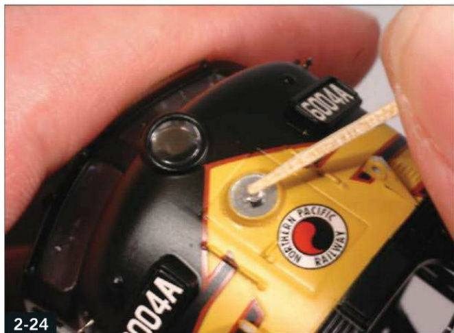
2-24 Add epoxy drop by drop to the headlight casting. Although not shown here, it's a good idea to cover surrounding areas with masking tape to avoid getting stray epoxy on the shell.
