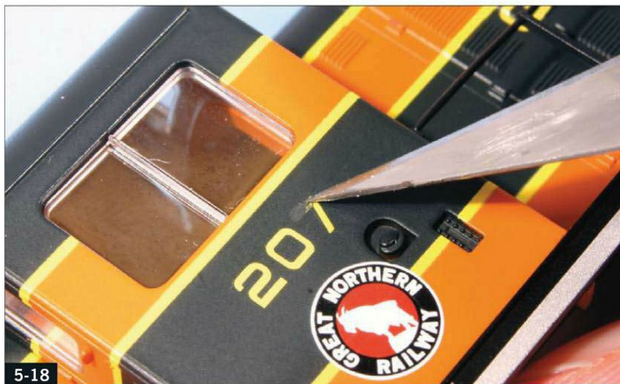
5-18 Use the tip of a hobby knife, laid flat, to scrape off the unwanted numeral.
