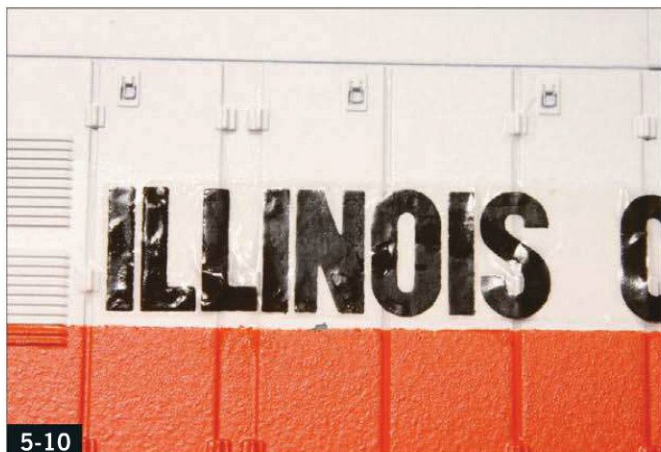
5-10 The decal will wrinkle as the setting solution goes to work, but it will lay flat when the solution evaporates.
