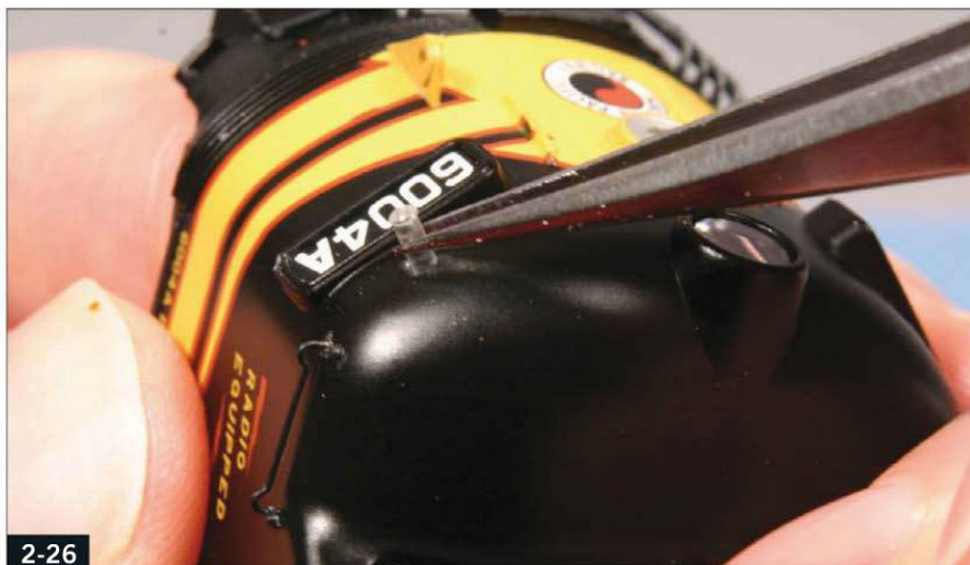
2-26 Drill a mounting hole for the class light using the model's bump as a guide, then glue the lens in place.
