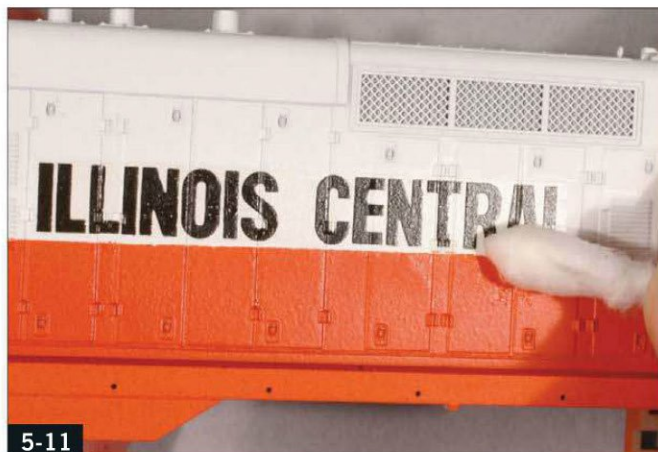
5-11 Once the decal is dry, wipe away any stains from decal solution with a damp cotton swab.
