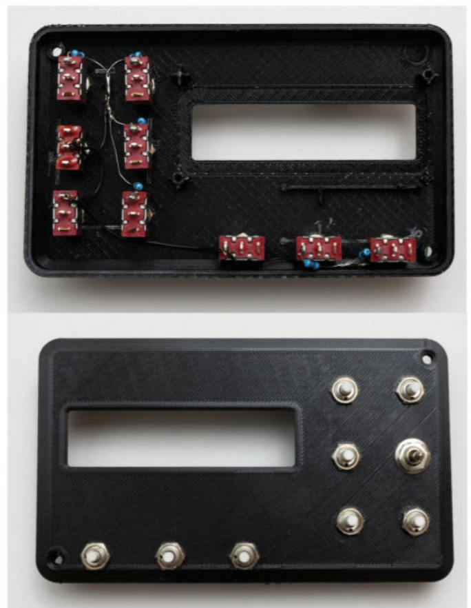
8 Add the switches to the case, and make the wire connections on the back.
