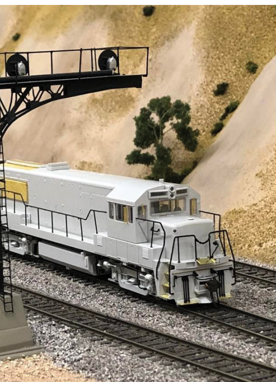
Above: Decoration on the Erie Lackawanna U25B provides the revised lettering style with yellow road name placed in the maroon band. Note the Radio Equipped logo and excellent rendering of a General Electric builder's plate on the area above the front truck.
