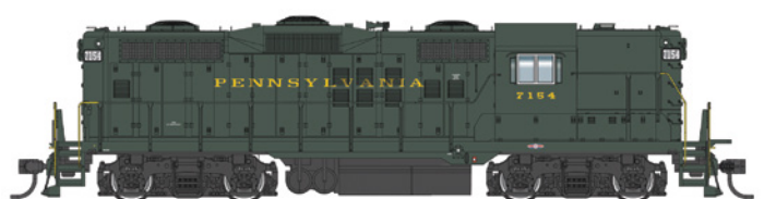
Above: A spotting feature differentiating EMD's Phase II GP9 production from the later Phase III offerings is the change from pairs of 36-inch fans on the roof (as shown on the Boston & Maine and Grand Trunk Western illustrations shown above at the left) to a single 48-inch fan as shown on the rest of the road names in this coming production. This Walthers Proto HO-scale GP9 diesel locomotive will come in standard DC version (MSRP: $199.98) and with ESU's LokSound 5 and DCC (MSRP: $299.98).
