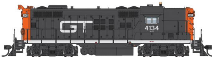
Above: A spotting feature differentiating EMD's Phase II GP9 production from the later Phase III offerings is the change from pairs of 36-inch fans on the roof (as shown on the Boston & Maine and Grand Trunk Western illustrations shown above at the left) to a single 48-inch fan as shown on the rest of the road names in this coming production. This Walthers Proto HO-scale GP9 diesel locomotive will come in standard DC version (MSRP: $199.98) and with ESU's LokSound 5 and DCC (MSRP: $299.98).
