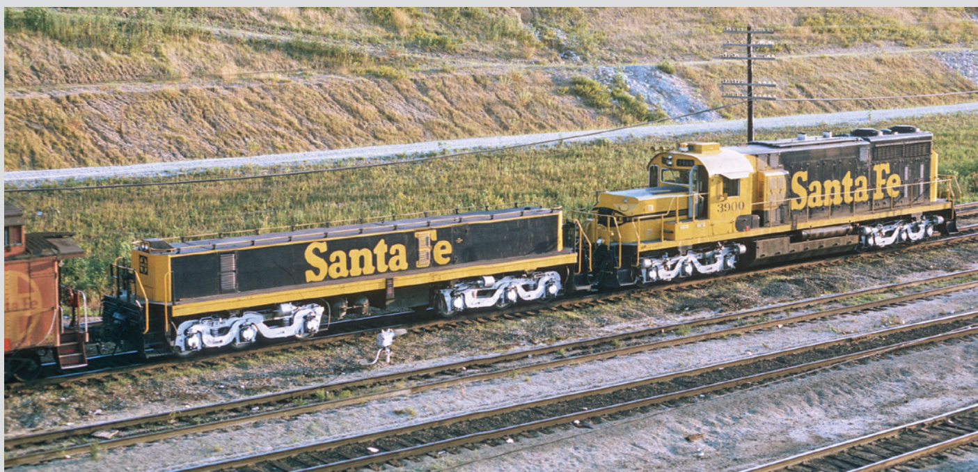
Above: If you're looking for a kitbashing project for your RSD-15, consider Santa Fe 3900, shown at Turner, Kan., in 1974. The road's RSD-15 delivered as 828 (later renumbered 9828), received an Electro-Motive makeover (note the fan arrangement on the roof of the long hood and grilles below those fans), and returned to service paired with a rebuilt RSD-5, becoming a set used in hump yard duty. Three Santa Fe RSD-15s (826 and 846 were the other two) and a trio of RSD-5 switchers were rebuilt in the 1970s. Santa Fe dubbed these units CRSD20 (3900–3902, renumbering in the late 1970s to 1300–1302). Another road to give new life to this type of Alco was Conrail, which recycled RSD-15s (along with RS-11 and RSD-12 roster members) into MT-4 slugs in the late 1970s. — James EuDaly photo
