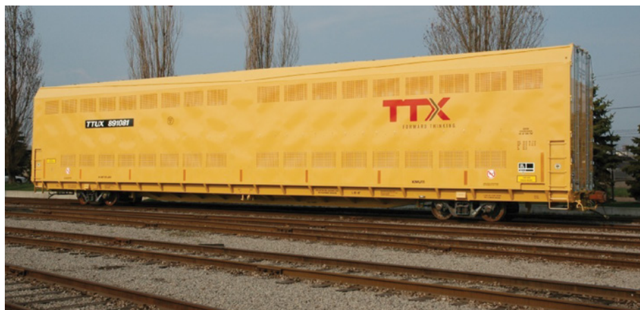
Above: This yellow Trailer Train car is an example of National Steel Car's uni-level autorack. This is a contemporary North American freight car that can handle transport of a variety of vehicles. — Norfolk Southern photo
