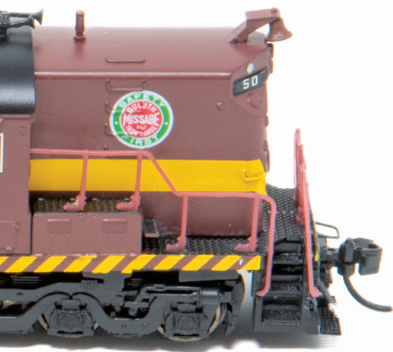
Left and Facing Page: The well-executed side-frames are plastic with a very good detail and dimensional depth to their appearance. The model, like the prototype, rides on 40-inch wheels. The flexible handrails come molded in color and include good stanchion detail replicating the prototype's design. Note the hoses, railing, and cut lever on the pilot.
