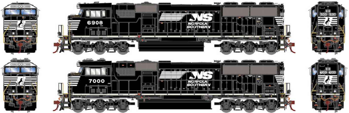
Above: Athearn will offer road-number specific detailing on its coming SD60E offerings. The illustration of NS 6908 shows an early version, while NS 7000 presents a later look for the SD60E. Compare the cab window styles and antenna details as spotting features differentiating the otherwise similar locomotives.
