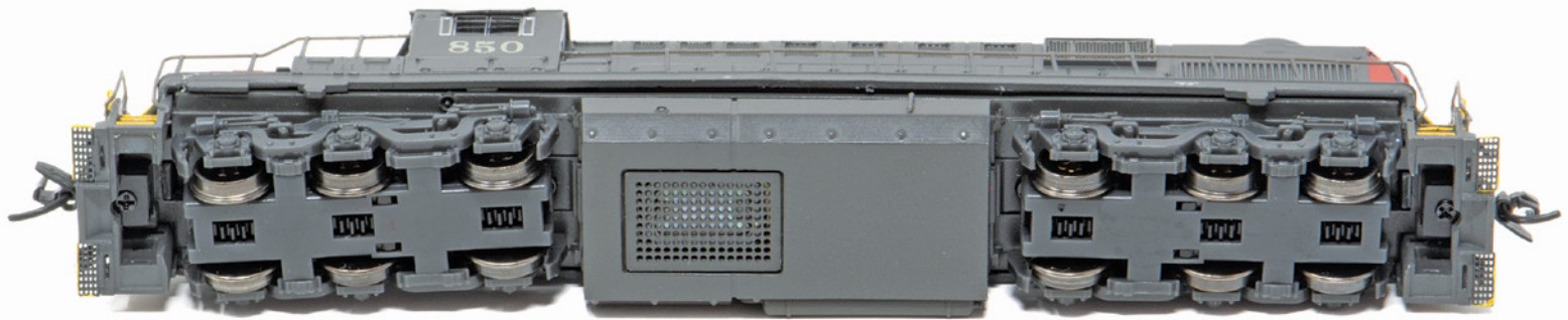
Above and Below: Working knuckle couplers are mounted to the locomotive's die-cast metal chassis. Once the couplers are removed, the plastic body shell will slide off the frame revealing the mechanism. The tanks are a separate, detailed plastic section with an opening on the base and an open grating covering the speaker (above). The footboards are see-through on the pilots and all axles are driven on this solid-performing N-scale Alco diesel locomotive. This run comes equipped with Paragon 4 electronics providing Digital Command Control and audio output.
