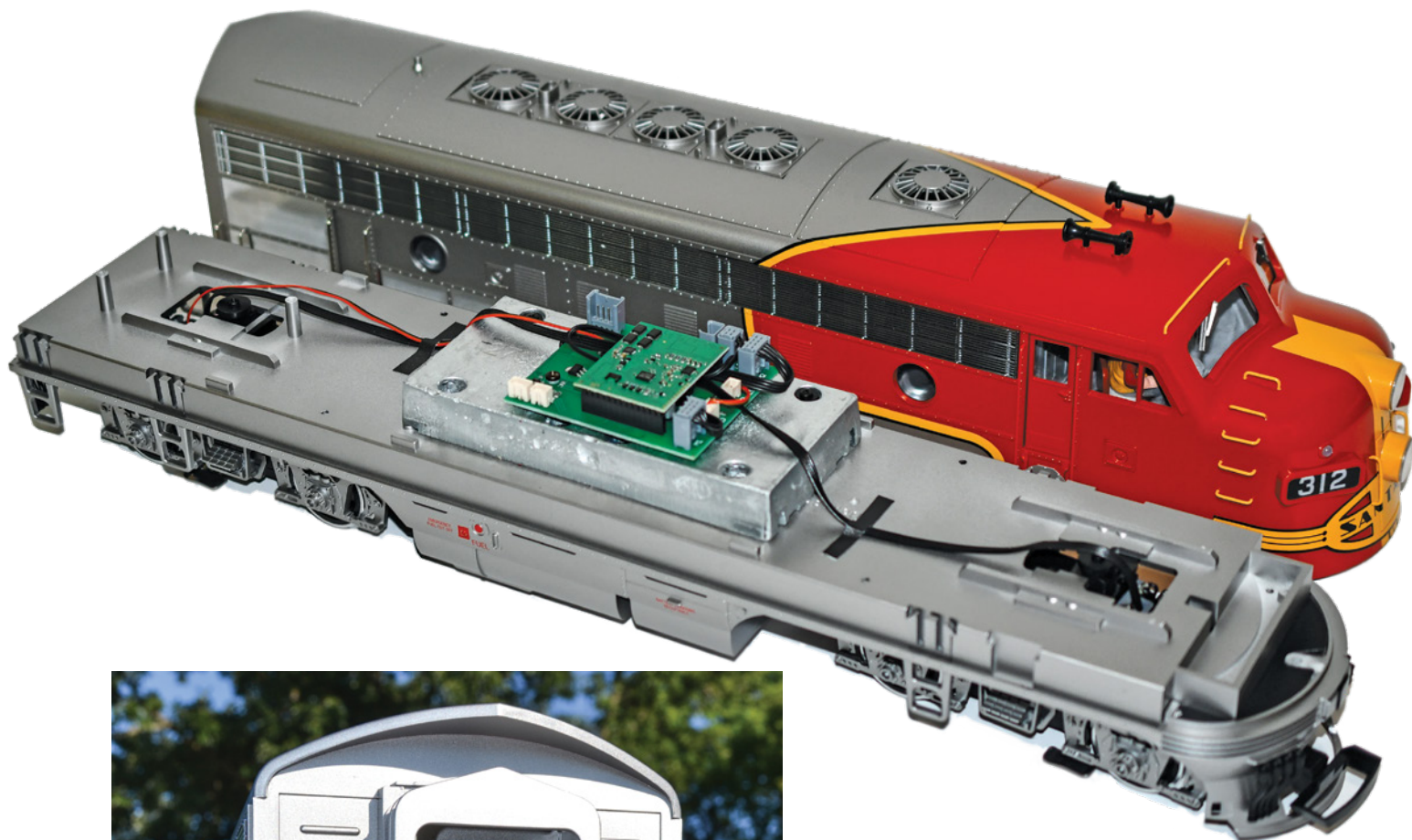
Above: LGB once offered an F7 with a clear body, we wanted to look under the hood on the DCC-equipped version. The main weight and DCC boards are in the center, with the wiring to each truck/motor block.
