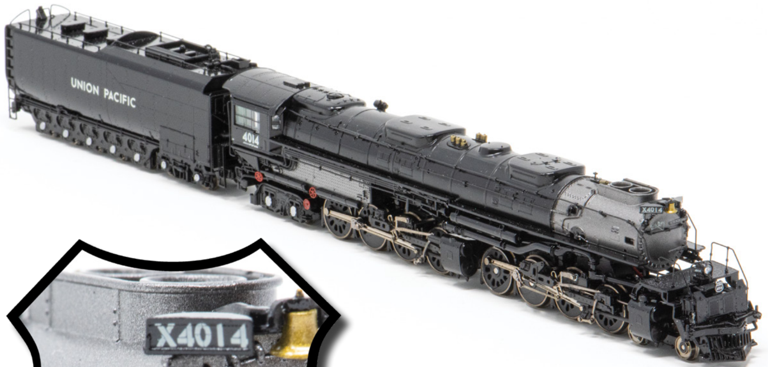
Above and Below: As delivered, Athearn's Big Boy includes a cover over the coupler area on the pilot. You can easily install a coupler (see pocket below behind the pilot) if you need double-header operations on your railroad.
