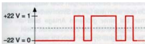
Quiescent levels Digital data Principal appearance of the digital tension at the track
