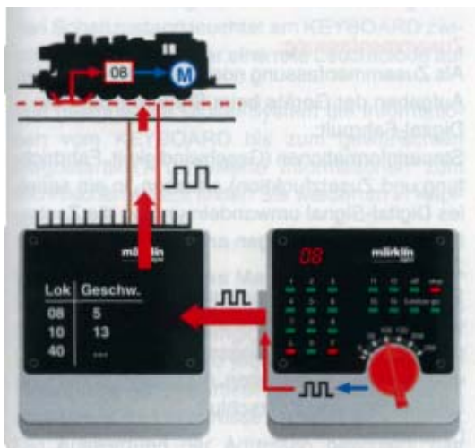
Central processing unit Control Panel
