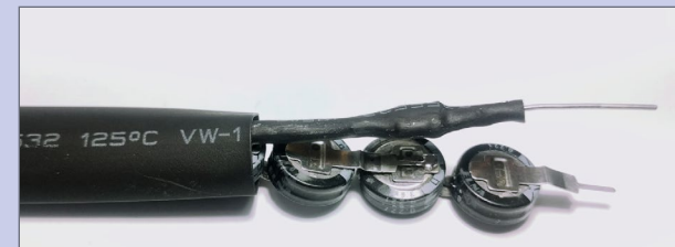
23. Shrink tubing installation.
