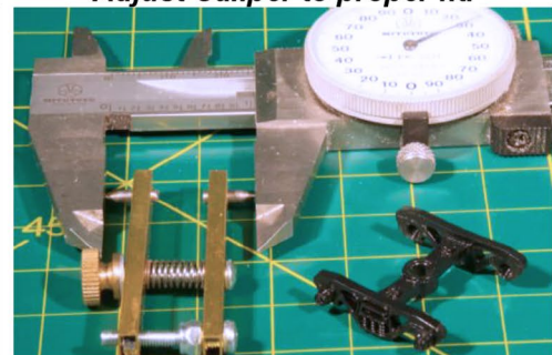
Measure for proper axle length.
