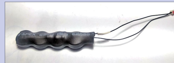
24. Assembled and ready to install StayAlive.
