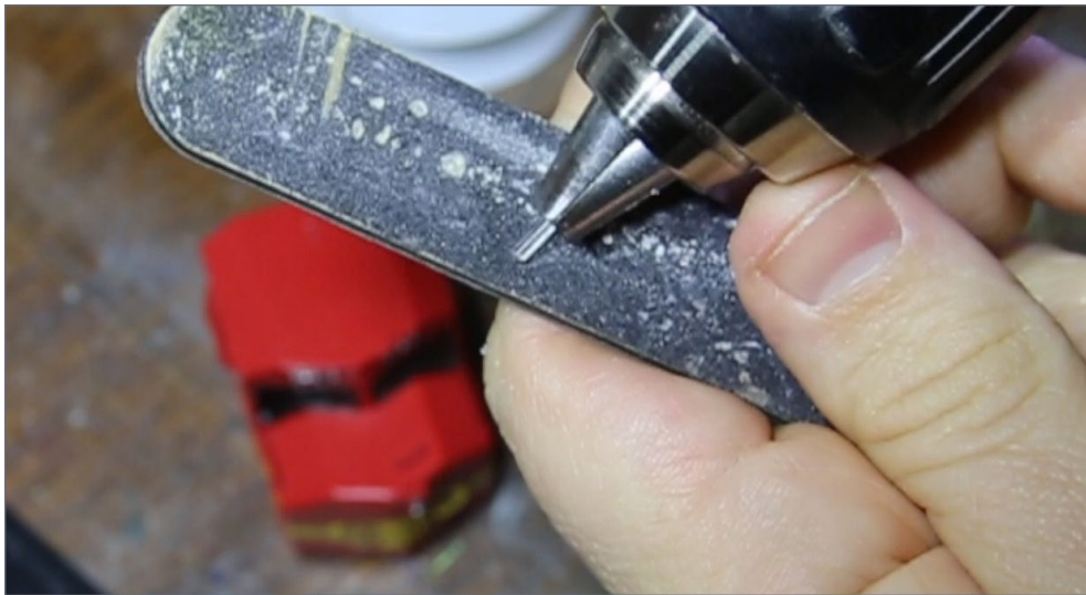
20. Lenses are shaped from acrylic rod against progressively finer grades of sandpaper.
