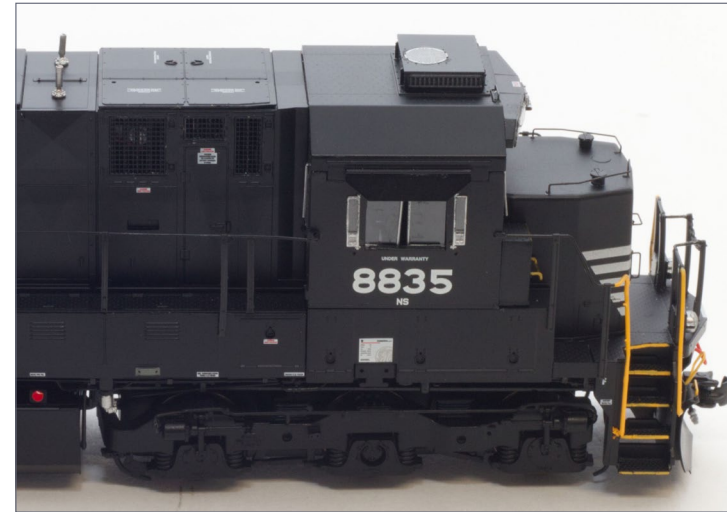
6. Engineer side, with the “Top Hat” AC and standard nose shape.
