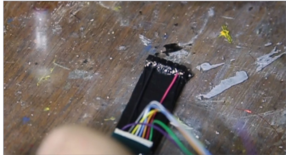
26. Red and black wire leads from this harness will connect to the decoder.
