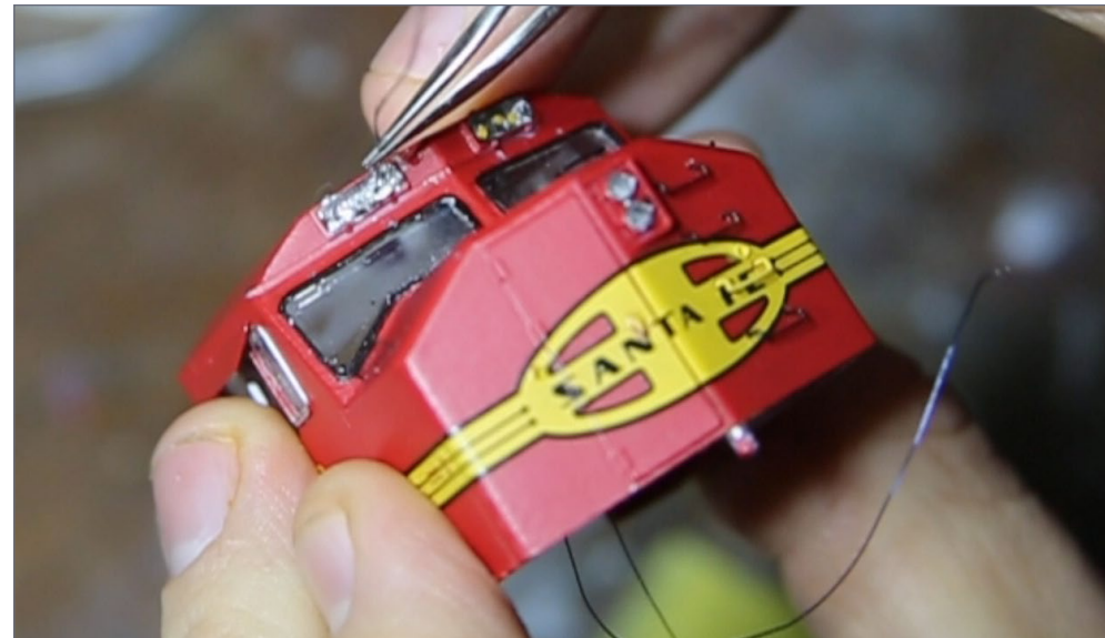
21. Each number board houses three LEDs, for even illumination.
