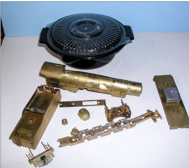
3. The model with some of the unwanted boiler detail unsoldered and removed. I went on to also remove the running boards, cab, boiler backhead, and smokebox front.
