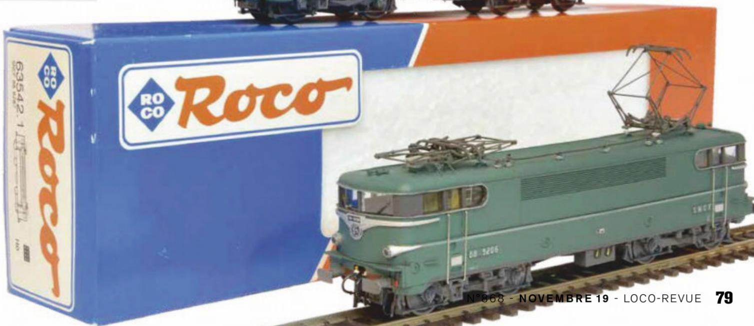
SUR SA BOÎTE, LA BB 9225 DE ROCO ; AU PREMIER PLAN, LA BB 9206 D'ATMOFER SUR CHÂSSIS ROCO.
