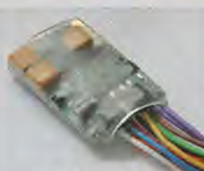
ZIMO MX648 20x11x4mm 6 Functions, 1W audio 0.8A Motor (continuous)
