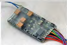
ZIMO MX645 30x15x4mm 10 Functions, 3W audio 1.2A Motor (continuous)
