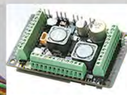
ZIMO MX695 50x40x14mm 8 or 14 Functions, 6Wx2 audio 10A Motor (continuous)
