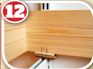
12 A spacer block is screwed into the bottom of the baseboard and strips of 1mm mounting card are added as necessary to ensure everything is totally horizontal. The whole process takes just a couple of minutes and allows any variations in the baseboard timber dimensions to be accommodated and compensated for.
