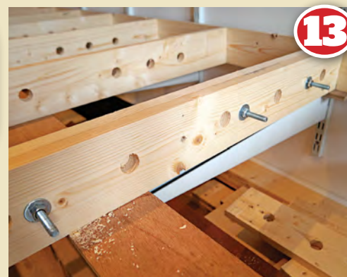
13 Before the adjoining baseboard section is fitted with spacer blocks it is bolted to its neighbour to ensure the accurate horizontal adjustments are maintained for the entire 16ft length of the wall.
