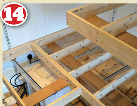
14 Corner section baseboards are bolted together and as each piece is added the entire level becomes more rigid. If planned properly then track sections could be removable allowing baseboard sections to be unbolted and removed if required.
