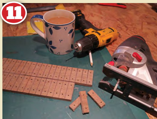
11 A batch of plywood spacer blocks are marked out of a spare section of plywood strip and then pre drilled ready to be fixed to the underside of the baseboards where they rest on the metal brackets.
