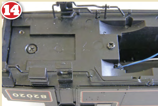
14 Rigidity was restored when the weight was fixed in place with the three screws and a few drops of cyano type adhesive in the relevant places. The body was set aside whilst the work moved onto preparing for the decoder and speaker installation.
