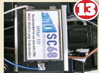
With a small blob of mastic I fitted the SC68 to this platform after soldering the blue and grey wires from the non harness end of the MX64SR. Polarity is important - blue to positive and grey to negative, as shown.
