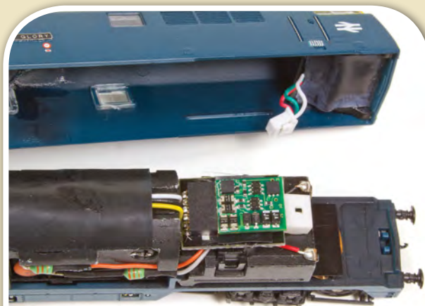
10 A 6-pin NEM-651 decoder plugs straight in its place. This is a Digitrax DZ126IN decoder.
