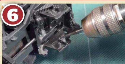
Now, with the finest cutting tool I could find, I drilled diagonally into the moulded axle bearings to deepen their coned ends. Only a small amount of material needs to be removed. There is no need to fit brass axle bearings as the slippery engineering-grade plastic from which the underframe is made presents a relatively friction free surface.
