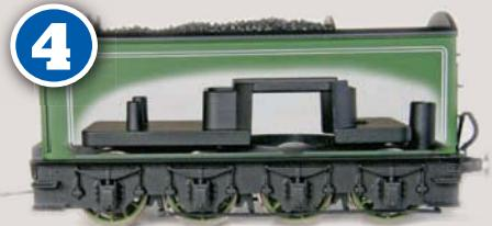
The cutaway view of the tender reveals that the chassis has been designed to house a speaker and most likely a sound decoder which will be populated by Hornby's TTS decoder in the production model.
