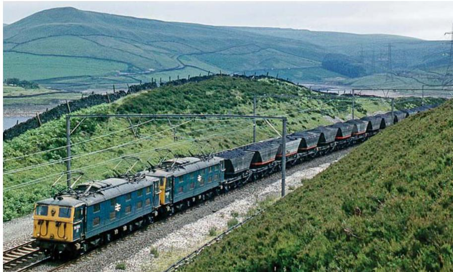
**The HAA coal hopper revolutionised coal traffic and made the only profitable component of freight traffic all the more efficient. On July 7 1981 EM1s 76034 and 76032 run downgrade past Woodhead Reservoir as they approach Torside with a westbound loaded MGR service formed of HAA hoppers. It was coal traffic which kept this route through the Pennines open into the 1980s.** Pete Berry/www.railphotoprints.co.uk.
