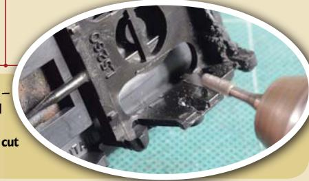
**5** To simplify fitting the replacement wheelsets – which are on 26mm axles – I opened out and deepened the vertical slots on the rear of the axleguards using a parallel burr. Be careful not to cut through to the front face!
