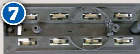
This mounting point is designed to accept a 28mm circular speaker and hold it clear of the chassis floor. In the non-sound fitted version it is an incomplete circular moulding with nothing to seal the speaker from the central channel in the tender chassis. I used sticky black mastic to fill the gaps and form a seal around the speaker. The rear gap is shown with mastic in place.
