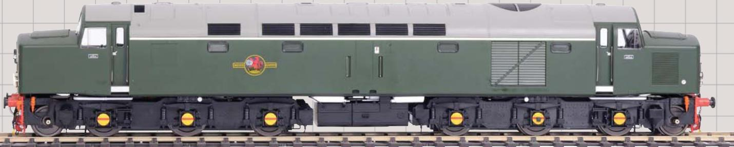
**T**HE CLASS 40 was typical of the early diesel era. Technology of the time meant that to produce the 2,000hp required English Electric's first production
