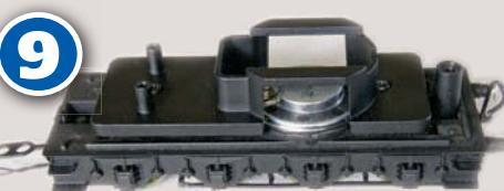
The ballast weight was refitted before remounting the tender body to its chassis – and there you go: a DCC sound model in just a few minutes. It really is that simple.
