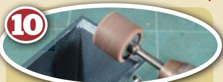
**10** The most obvious failing of the moulded bodywork is the broad, thick ledge at either end – on the real thing, this is quite a narrow lip. I took this off with a sanding disc in my Dremel, finishing off with progressively finer emery boards.
