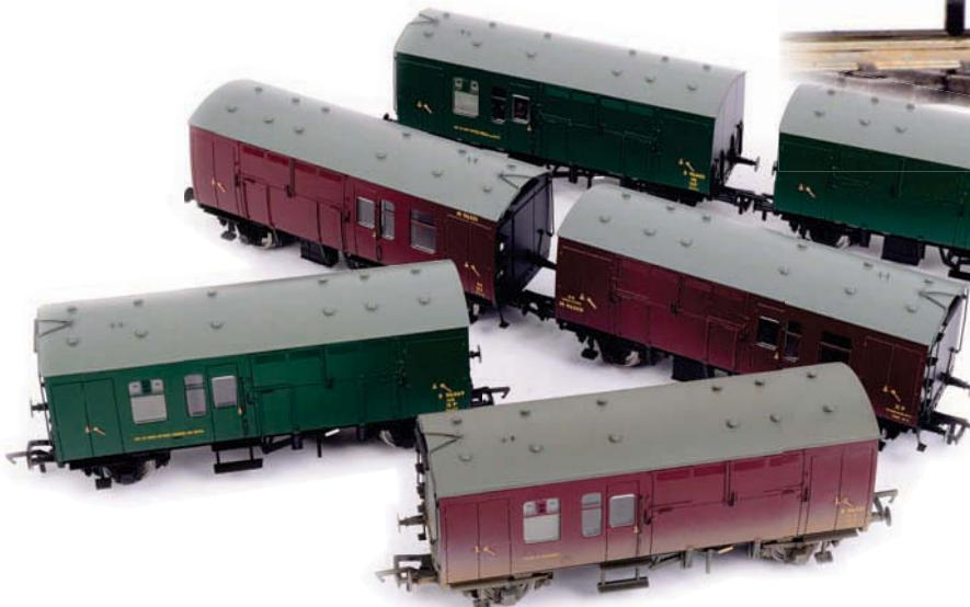
they now feature strengthening bars on the side doors and/or ends - a development of the prototype whilst in service.
