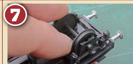
By bending one axleguard outwards while you locate the pinpoint at the other end of the axle, the new wheels should slip comfortably into position. If they don't spin easily, remove more plastic from the coned bearings. The replacement white metal buffers came from Lanarkshire Model Supplies (Oleo pneumatic buffer BP03).
