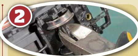
Real HAA wagons ride around on 3ft 6in diameter wheels of two distinct patterns. Hornby's plastic wheels are too small, so the wagons ride at the wrong height. I got rid of them by cutting through the axles with a wire cutter – there's no chance these wheelsets will be reused on another wagon.
