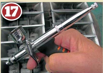
With the exteriors of 32 wagons to weather I needed an airbrush that could deliver a high volume of paint and yet remain controllable down to the gentlest waft. My choice was the trigger-operated Iwata TRN-2, my favourite airbrush for all high volume work. The pistol grip ensures the airbrush is comfortable to handle over long sessions.
