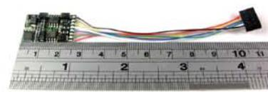
10231-01 8-pin 3-function 1-sided 1/1.8A decoder (Outputs A, B & C) (Len) ..... £18
