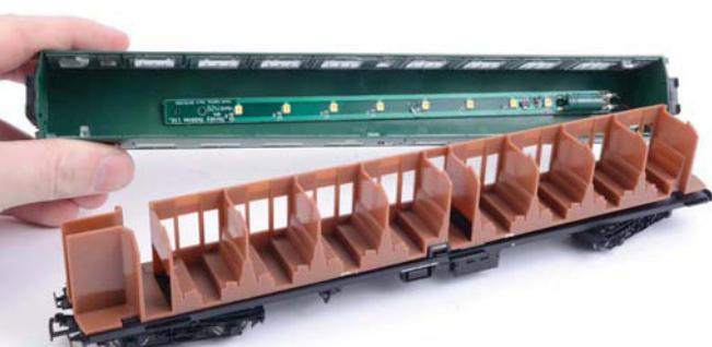
An LED lighting strip mounted to the roof lights the Mk 1s interior.
