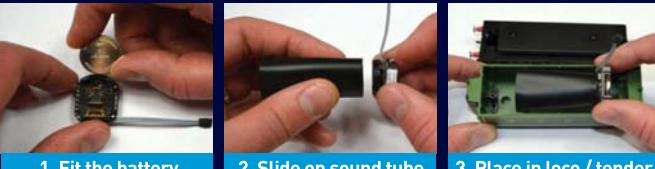
1. Fit the battery    2. Slide on sound tube    3. Place in loco / tender
