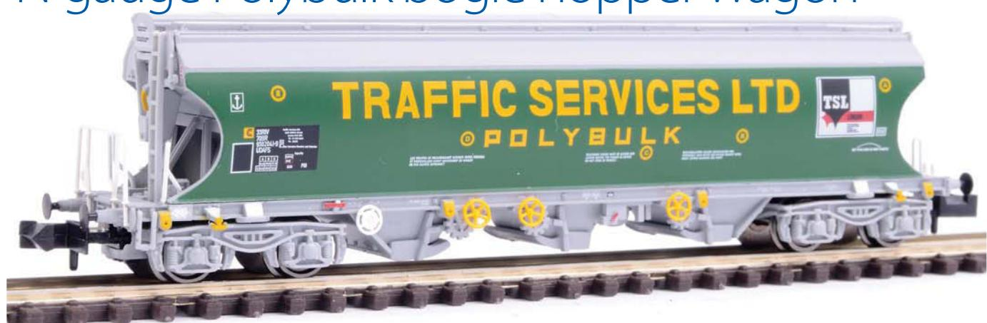
The eagerly awaited 'N' gauge model of the Polybulk covered hopper wagon from Bachmann's Graham Farish range is here. Built by Fauvet Girel of France in the 1970s, these wagons could be seen operating across the British Rail network.
