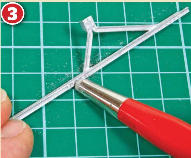
Each casting was given a gentle rub down with a glass fibre pencil to remove tarnish and casting flash before assembly.
