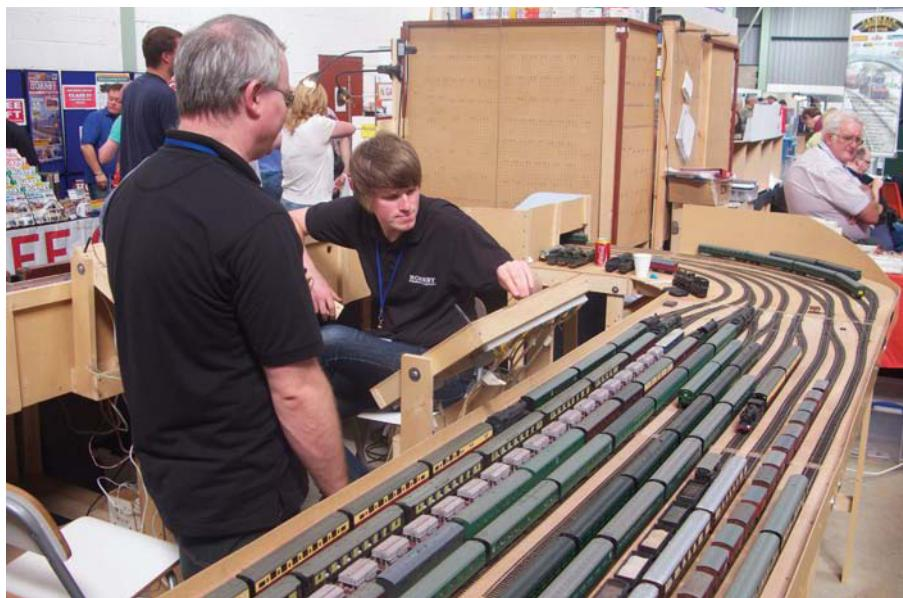
Ladder fiddle yards can be built in a number of ways. This is the ladder yard for *Hornby Magazine's* Bay Street Shed which featured a central reversing road and a trio of sidings to the rear for multiple unit storage.
