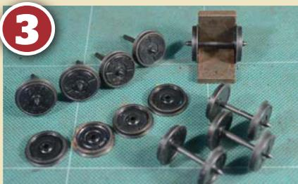
Because of the complicated brake arrangements of these wagons, they have mixed wheelsets – viewed side on, the arrangement features disc brake wheels at the left-hand end and plain disc for the clasp brakes at the other. I bought 32 sets of Alan Gibson's 14mm disc brake wheels (4013) and 32 axles' worth of 14mm plain disc (4005). I redistributed them so each axle had a disc brake wheel on one side and a plain disc wheel on the other. Using a back-to-back gauge ensures dimensional accuracy.
