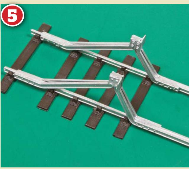
Sleepers are fitted to the bufferstop sides with the flange of each frame assembly facing out. A piece of styrene card can be cut to size and used as a spacer to keep the side assemblies apart when fitting the buffer beam.
