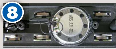
I used a thin bead of mastic to hold the speaker in place and form a seal. The sound from the front of the speaker will escape though holes for the wheels and the tender body will become the speaker enclosure when refitted. The extended speaker wires were fed through to the speaker and soldered in place.
