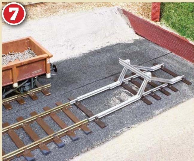
Installation commences by measuring exactly where the bufferstop is to fit and laying the siding track up to that point.
