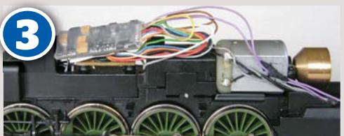
I loosely coiled the decoder leads to shorten the overall length of the harness and plugged in the decoder. In this case I used a Zimo MX645R sound decoder, but other decoders would fit in a similar way. I ran the speaker wires to the rear of the chassis, extending them with thin black wire to bridge the gap between locomotive and tender, where the speaker will be situated.
