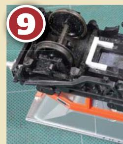
**9** You can do the same at the other end, or you can make a framework of 60 thou styrene strip so the axle unit is allowed to rock but not to pivot. With this modification to a three-point suspension system, the wagons ride much better, especially on curves.
