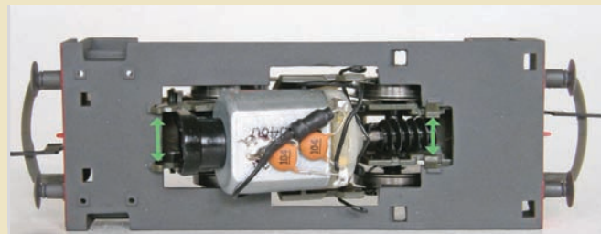
4 That's all the work needed to commence the installation, but if you wish to separate footplate casting from chassis, ease out the tabs arrowed in green.
