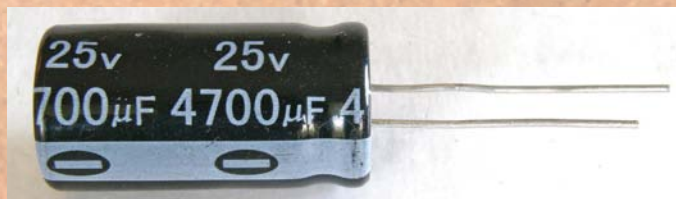
Above: Here's the essential information you can derive from each capacitor: The working voltage - 25V. If too low you risk explosion. If too high it is safe but less efficient. The capacitance - 4700 microFarads, or 0.0047 farad. This figure shows the maximum storage, the 'µ' is a Greek letter used to denote 'micro' or 'one millionth part'. The F is the symbol for the farad, the unit of capacitance. The larger this figure, the more energy may be stored.
