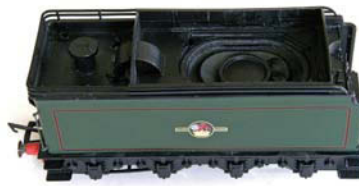
Figure 3: Single speaker installation in a Hornby 'A3' tender.
