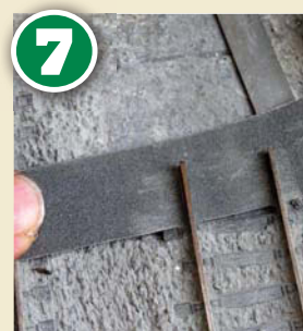
As the first stage in cleaning up the old track for soldering, a piece of emery paper can be slid under the rails and used to clean the underside for attaching a copper paxolin sleeper. The side of the rail can quickly be cleaned with a small dentist's grinding bit ready for electrical bonding.
