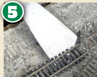
As the first stage in cleaning up the old track for soldering, a piece of emery paper can be slid under the rails and used to clean the underside for attaching a copper paxolin sleeper. The side of the rail can quickly be cleaned with a small dentist's grinding bit ready for electrical bonding.
