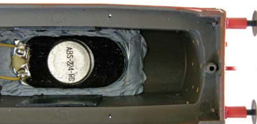
Figure 8: This Bachmann Class 20 has a 'tortured' sound path created by sealing it to the roof with Blu Tak. The rear waves then escape through the chassis and bogies enhancing the sound effects.
