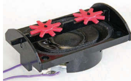
Figure 9: Produced exclusively for Rail Exclusive's ViTrains Class 47s, this laser cut speaker support mounts directly into the locomotive body and also supports the roof fans.
