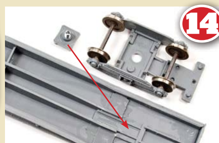
Another view of the bogie pivot in relation to the underframe trussing. The bogie, when test fitted, must clear the 'fish-belly' frames, so be careful to glue the pivots in the correct place.
