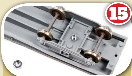
The wagon is test assembled at regular intervals as dry runs before applying solvent cement. Should I make a mistake I have a good chance of correcting it before moving too far along in the building process.
