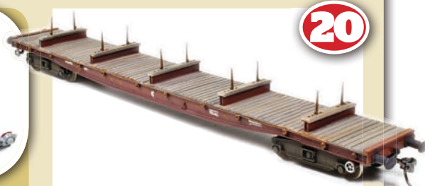
The 'Borail' was finished as a vacuum braked wagon painted in pre-1982 condition. The livery is bauxite with white lettering and black bogies with rust grime and dirt applied.
