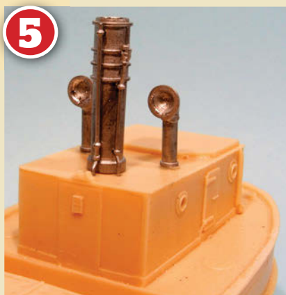
In front of the wheelhouse we have the funnel and two larger vents. These normally face forward but this varied between boats.
