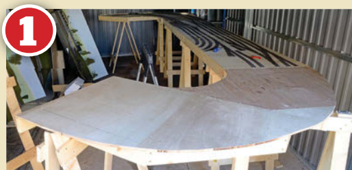
The first step in modifying the station end of the fiddle yard was to build a new bespoke baseboard to link with the scenic section. It has been made with 69mm x 20mm timber for the frame and 9mm plywood for the surface.
