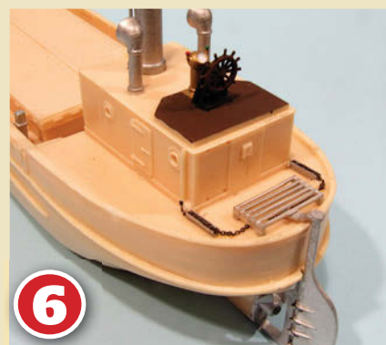
Puffer steering is simple. A chain attached to the tiller (lever attached to the top of the rudder) runs up either side of the engine room and on to the back of the wheel. You could model the whole set-up but we ignored the hidden parts inside the wheelhouse.
