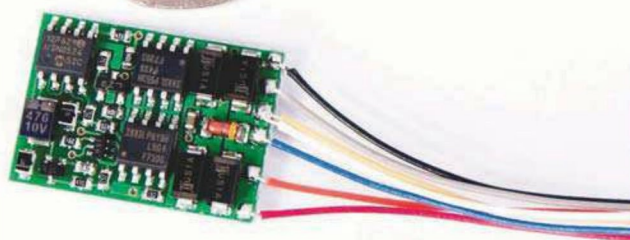
This is a Lenz LE1000E decoder chip. On the left is the decoder chip which communicates with the controller, while at the other end of the wires is the plug which connects to a standard 8-pin decoder socket. Mike Wild.
