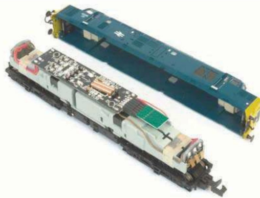
Although 'N' gauge models are now being fitted with tabs to solder a 6-pin decoder to, space is still at a premium inside – a necessary evil of adding enough weight to allow adequate haulage capacity. Mike Wild.
