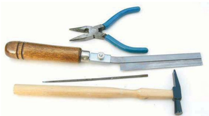
A selection of tools is essential to create the best possible trackwork. From the top: pliers, a hacksaw (or electric mini-drill with a cutting disc), a small file and a pin hammer.
