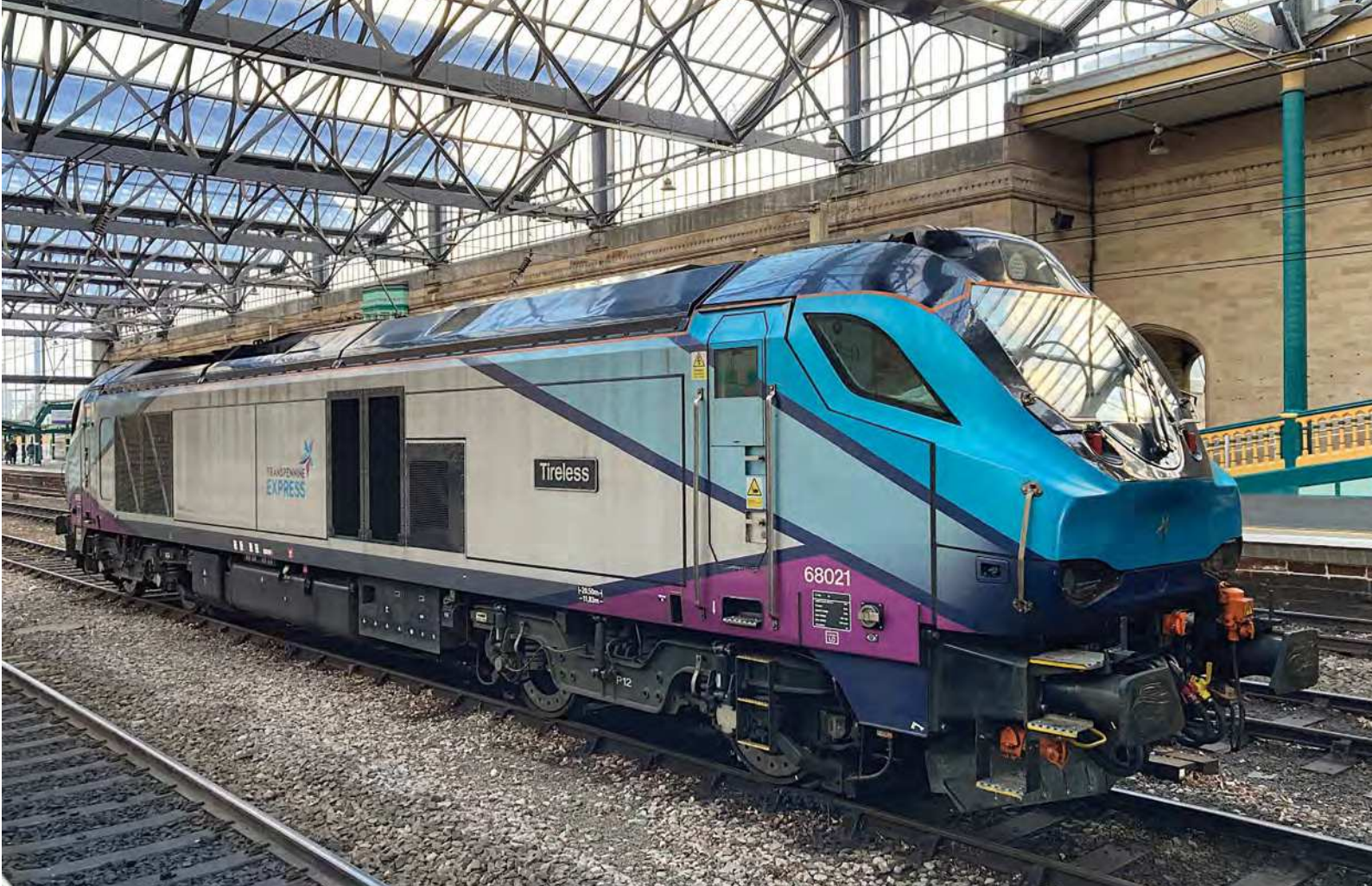
TransPennine Express liveried Class 68 68021 Tireless rests between duties at Carlisle station. Note the subtle streaking down the bodysides which appear to match the line of bolts along the cantrail. Andy Glover .
