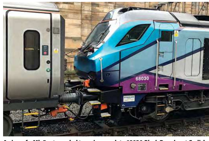
A view of a Mk 5 set coupled to an immaculate 68030 Black Douglas at Carlisle station. Just look how many pipes and cables are connected to the Class 68. Andy Glover .
