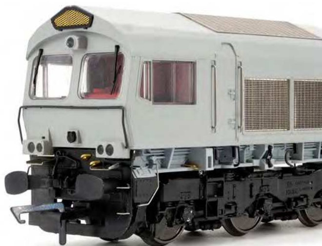
A raft of refinements have been introduced to enhance the appearance and running characteristics, including revised rotating axleboxes.
