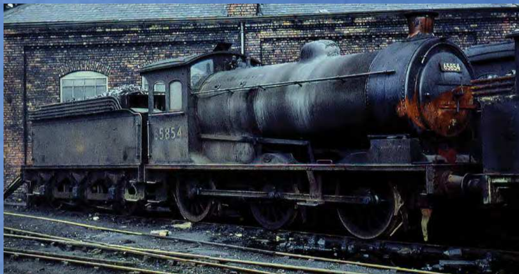
Seen at its home shed of Sunderland on July 24 1960, 65854 shows evidence of hard work and a fair bit of priming. There are big problems with the smokebox, which has recently been repainted after repairs. Already the door is badly burned and so is the chimney. Jacy collection.
