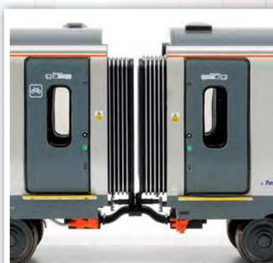
Magnetic couplings are fitted between vehicles on the Mk 5a coaches with small tension locks at the outer ends. Close coupling is impressive on straight track.
