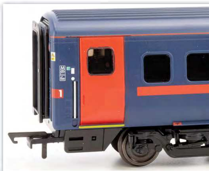
Below: The Swiss SIG BT41A bogies replicate the real vehicles well and are fitted with turned metal wheels.
