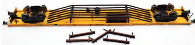
Detailing includes underfloor trusses, storage compartment and fine pipework on the air-braked example of the 'Salmon'.
