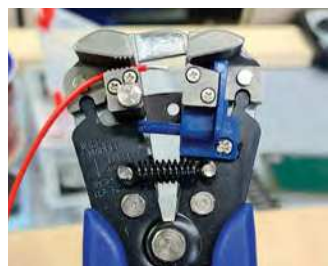
Preparation of the layout bus wire requires removal of a small section of the protective insulation. We used a DCC Concepts power bus stripper.
