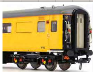
The non-driving end features TDM cables for connection through the train to the locomotive for push-pull working.
