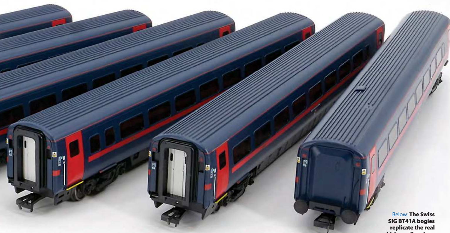
The coupling bar clips into the NEM pocket on each coach and still allows the vehicle to negotiate second radius curves.
