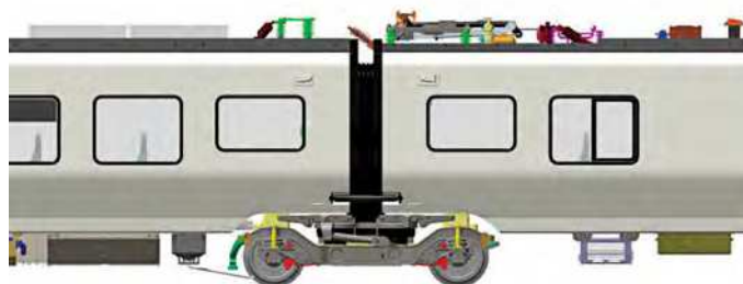
Below: A distinctive feature of the full-size prototype is the shared bogie design between vehicles.
