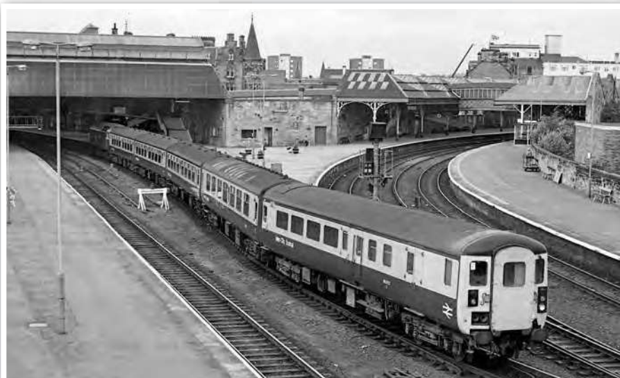
The second batch of Mk 2F DBSOs were built to work with Mk 2 coaching stock for push-pull trains to Aberdeen. On August 29 1984 Class 47/7 47701 propels a service for Edinburgh out of Perth led by DBSO SC9709. John Chalcraft/Railphotoprints.uk.
