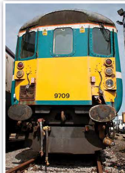
Following the derailment at Polmont in 1984 the DBSO fleet were fitted with obstacle deflectors beneath the leading buffer beam. This is withdrawn Anglia Railways DBSO 9709 at Eastleigh on May 23 2009. Colour Rail.
