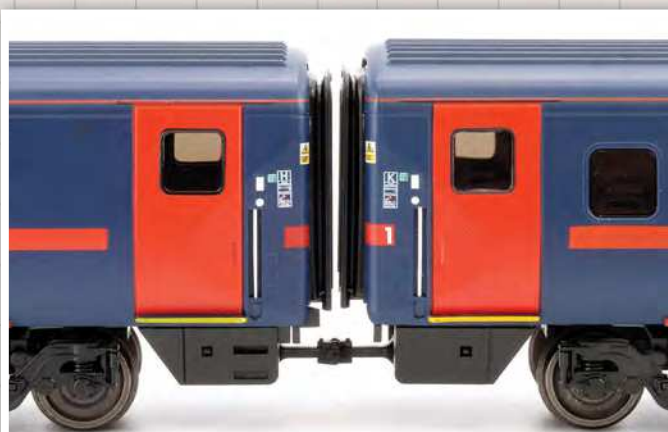
Optional close coupling bars are included with each coach and they make a big difference to the appearance of these coaches on the track.
