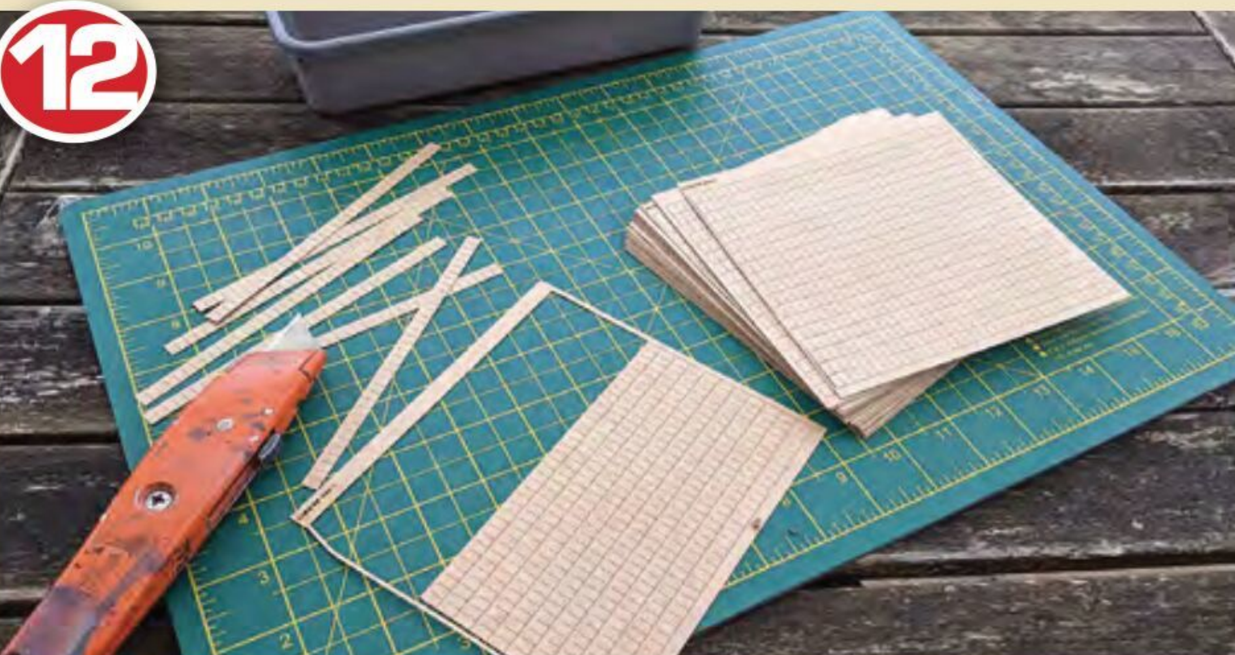
With a large engine shed comes a large roof, requiring a great deal of roof tiles to complete the structure. A methodical approach is required here. I used a sharp craft knife, slowly releasing the tile strips from their frets section by section.
