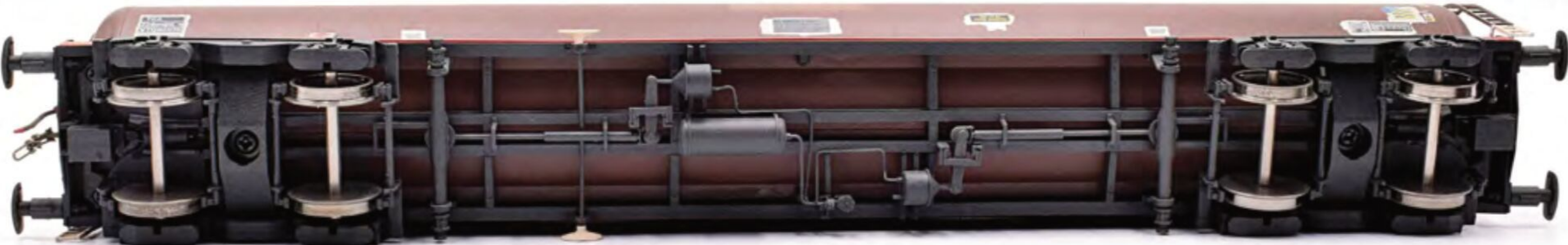
The underframe is neatly appointed with refined bogies, brake shoes in line with wheels, brake and discharge equipment.
