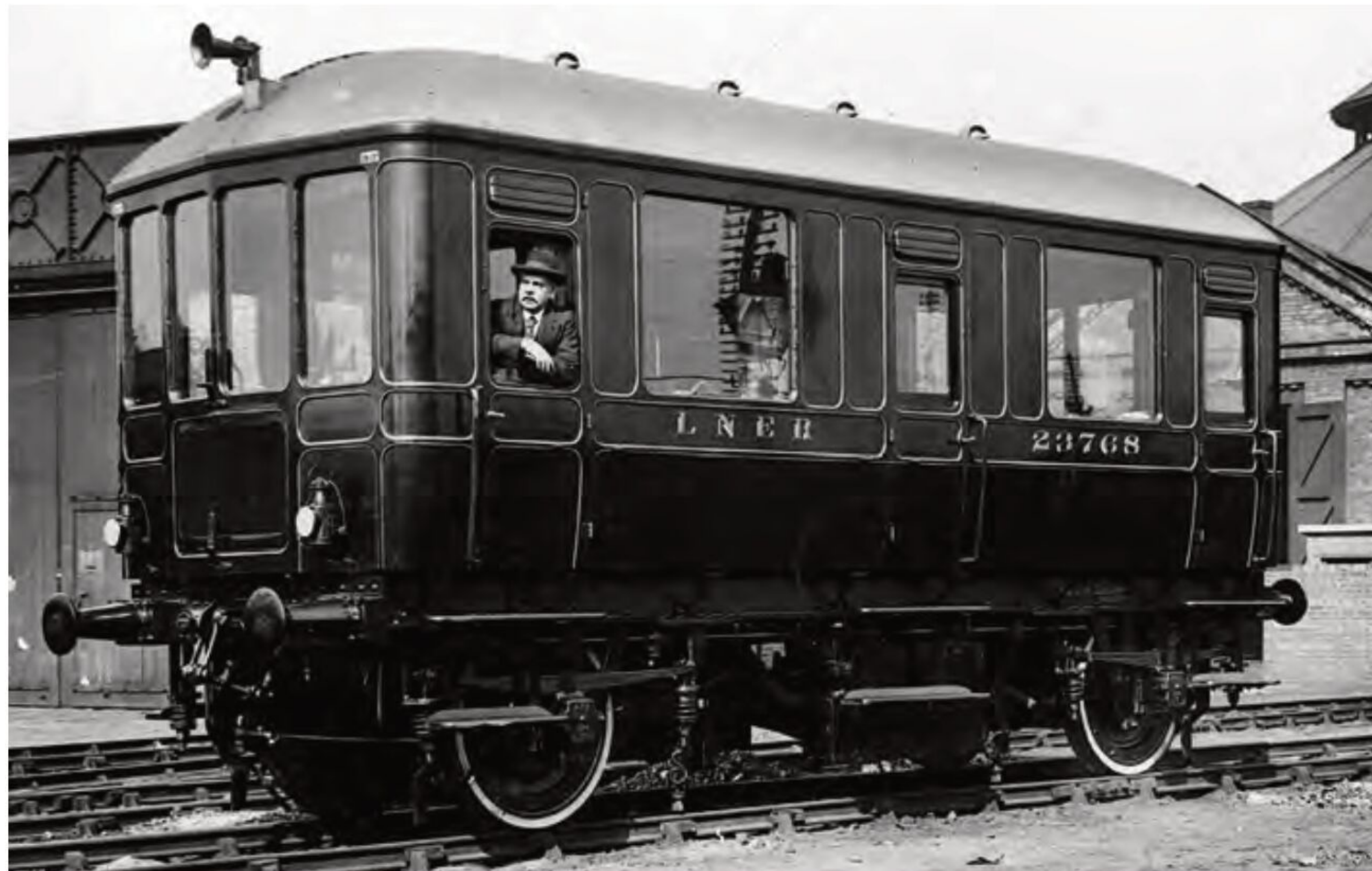
The LNER built a petrol powered inspection vehicle, 23768, in 1931. It had a four-wheel chassis. Getty Images.
