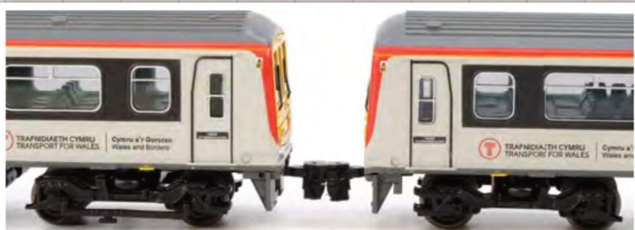
Realistic functional ‘push-fit’ couplings are fitted to the outer ends of each four-car set to enable multi-unit formations to be created.
