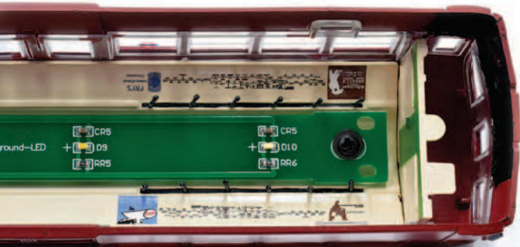
The carriage roof interiors have superb printed route maps and period adverts as well as LED lighting.
