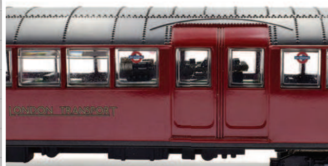
PluX22 decoder sockets are fitted into each Driving Motor car, but they are visible through the windows, particularly once a decoder is fitted as here.
