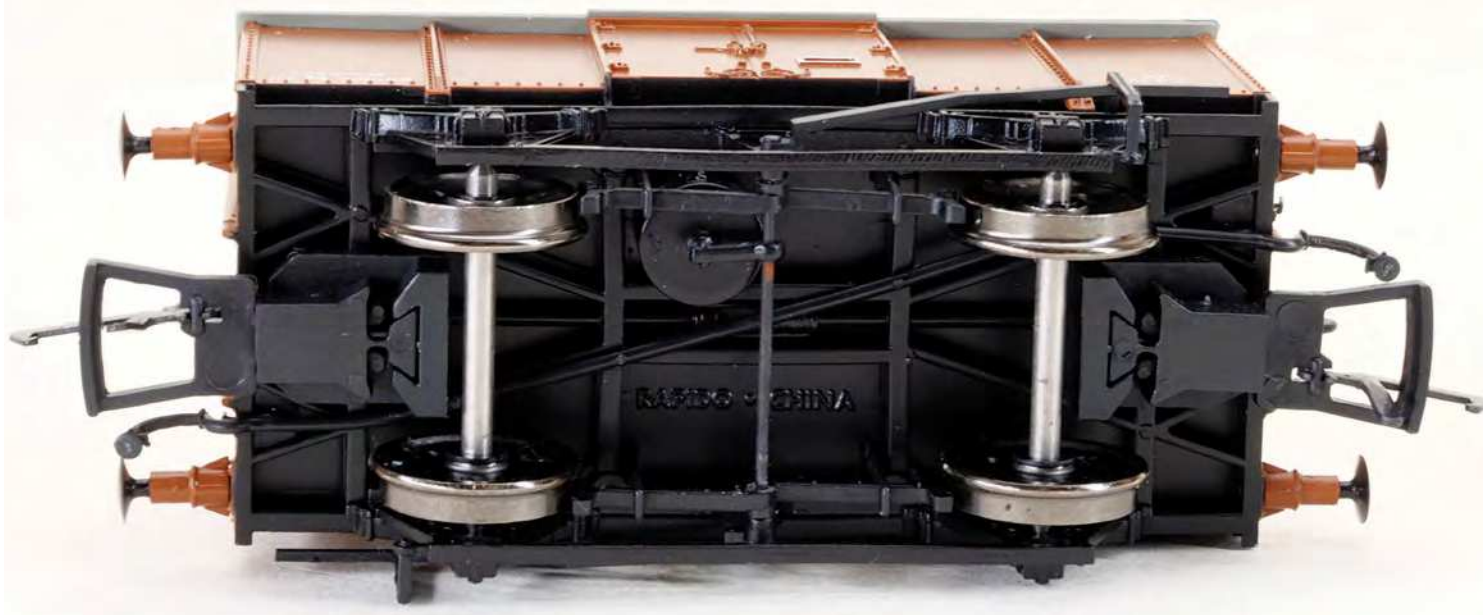
The underframe of the BR vacuum fitted wagon features a full length brake pipe.
