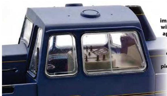
Hornby's all-new Sentinel incorporates pick-ups to all wheels and drive to the centre axle.
