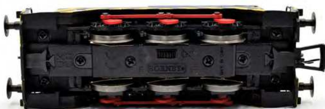
Hornby's all-new Sentinel incorporates pick-ups to all wheels and drive to the centre axle.
