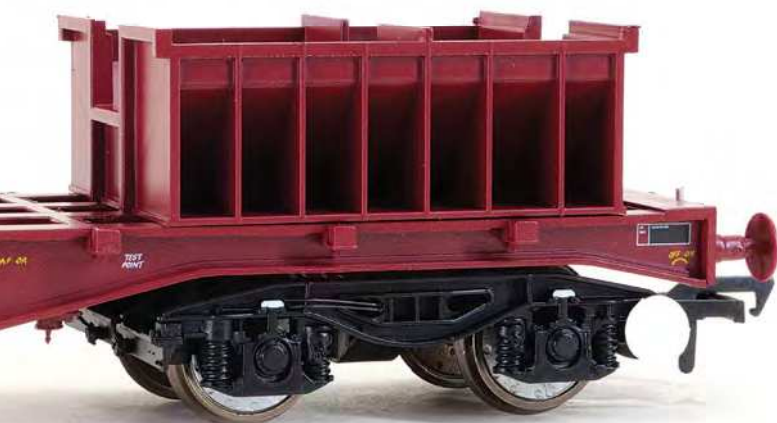
The BLA coil wagons feature correct cradles and detailed bogies.
